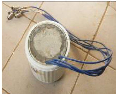
Fig. 1. Schematic illustration and specimen of concrete used for the humidity testing.
