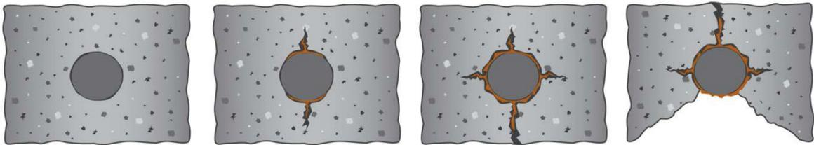
Fig. 7. Development of corrosion of a reinforcement bar in concrete.
