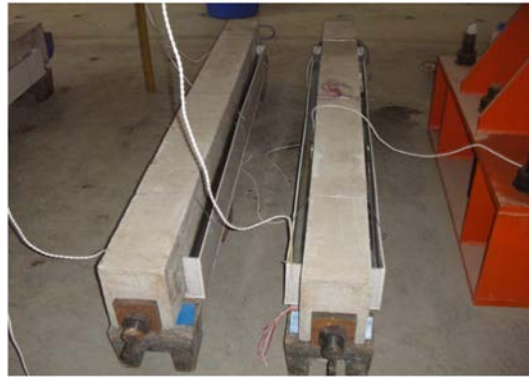
Fig. 6. Accelerated corrosion test of beams.
