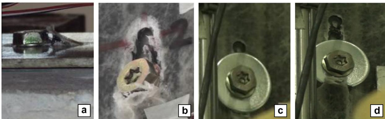
Fig. 6. DST-1 (a and b) and DST-1w tests (c and d): main damage mechanisms.
