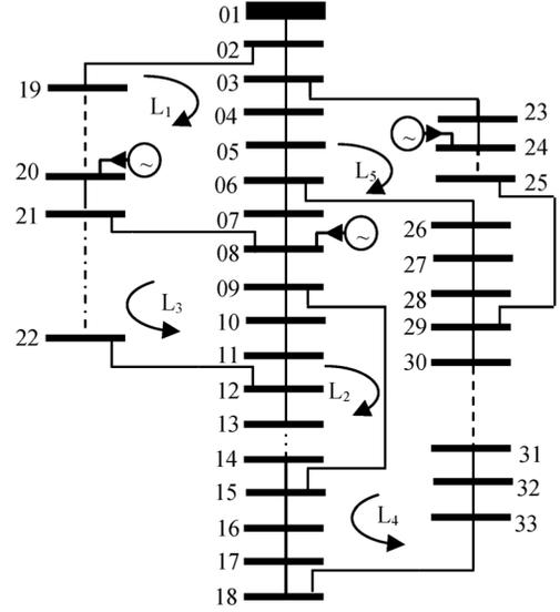
Fig. 4. 33-bus radial distribution system for  $HV^2$ .
