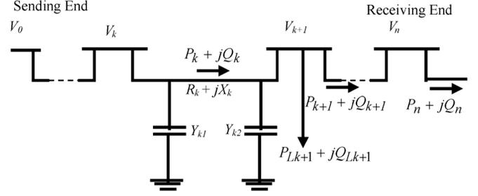
Fig. 1. Single-line diagram of a main feeder.
