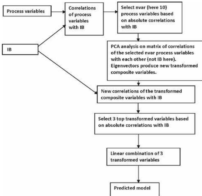
Figure 1. — Flowchart of Modified Principle Component Analysis approach.
