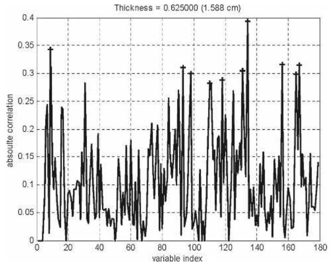
Figure 2. — Absolute values of the correlations of process variables with IB for thickness of 0.625 inches (15.88 mm) where the top 10 are marked as crosses.
