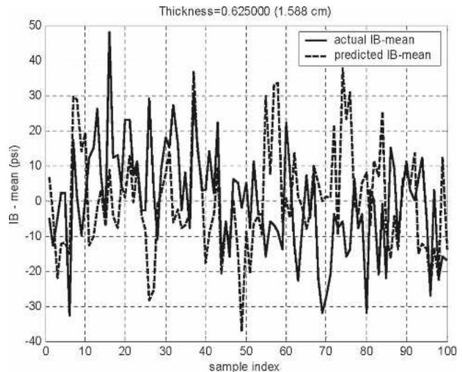
Figure 4. — Observed internal bond with mean IB subtracted and predicted IB with mean subtracted from first dominant transformed composite variable for thickness of 0.625 inches (15.88 mm).
