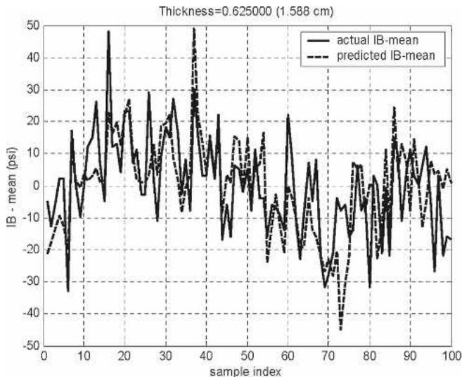
Figure 5. — Observed internal bond with mean subtracted and predicted IB with mean subtracted from linear combination of all three dominant transformed composite variables for thickness of 0.625 inches (15.88 mm).
