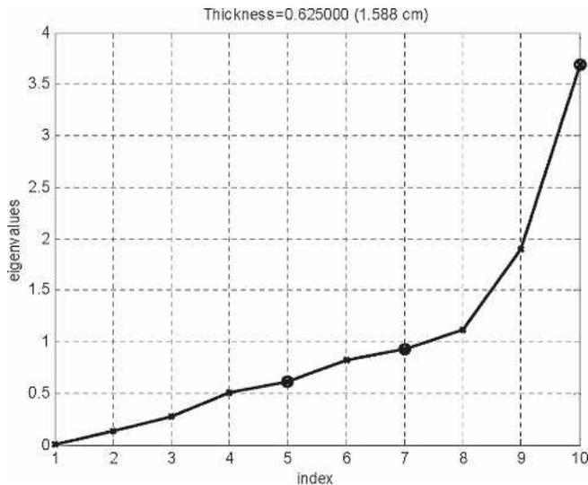
Figure 3. — Ten eigenvalues for process variables shown in Table 1 for thickness of 0.625 inches (15.88 mm), larger dots are for the associate transformed composite variables with the higher absolute correlations with IB with their associated indices are later relabeled as 1 (highest), 2, and 3 respectively.
