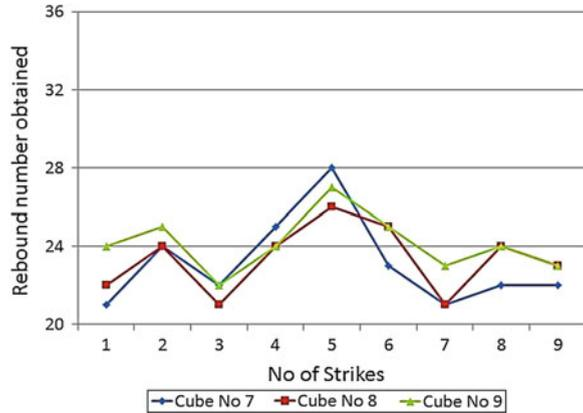
**Fig. 6** Rebound numbers achieved for cubes damaged at 1,100 °C
