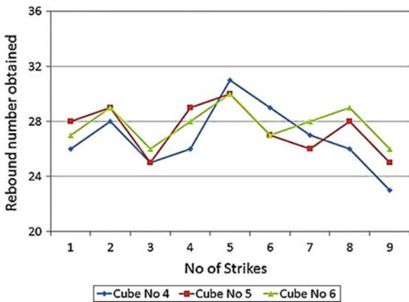
**Fig. 5** Rebound numbers achieved for cubes damaged at 500 °C
