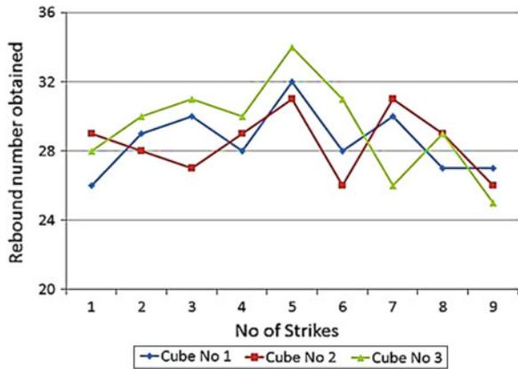
**Fig. 4** Rebound numbers achieved for cubes damaged at 250 °C
