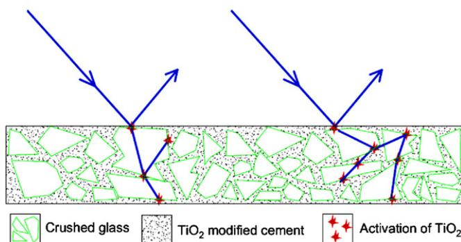
**Fig. 4.** Pathways of light and activation of TiO<sub>2</sub> in concrete block surface layer using glass as aggregates.
