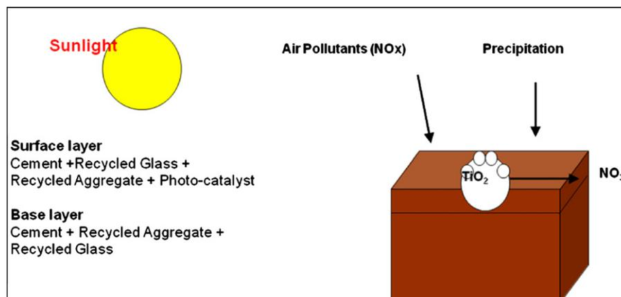
Fig. 3. Two-layer block structure prepared with different ingredients.
