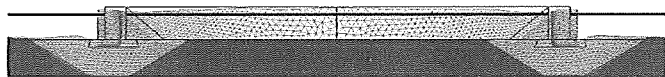
Figure 26 Deformed mesh at the end of the earthquake ( t=30 s) when tied degree of freedom boundaries are used
