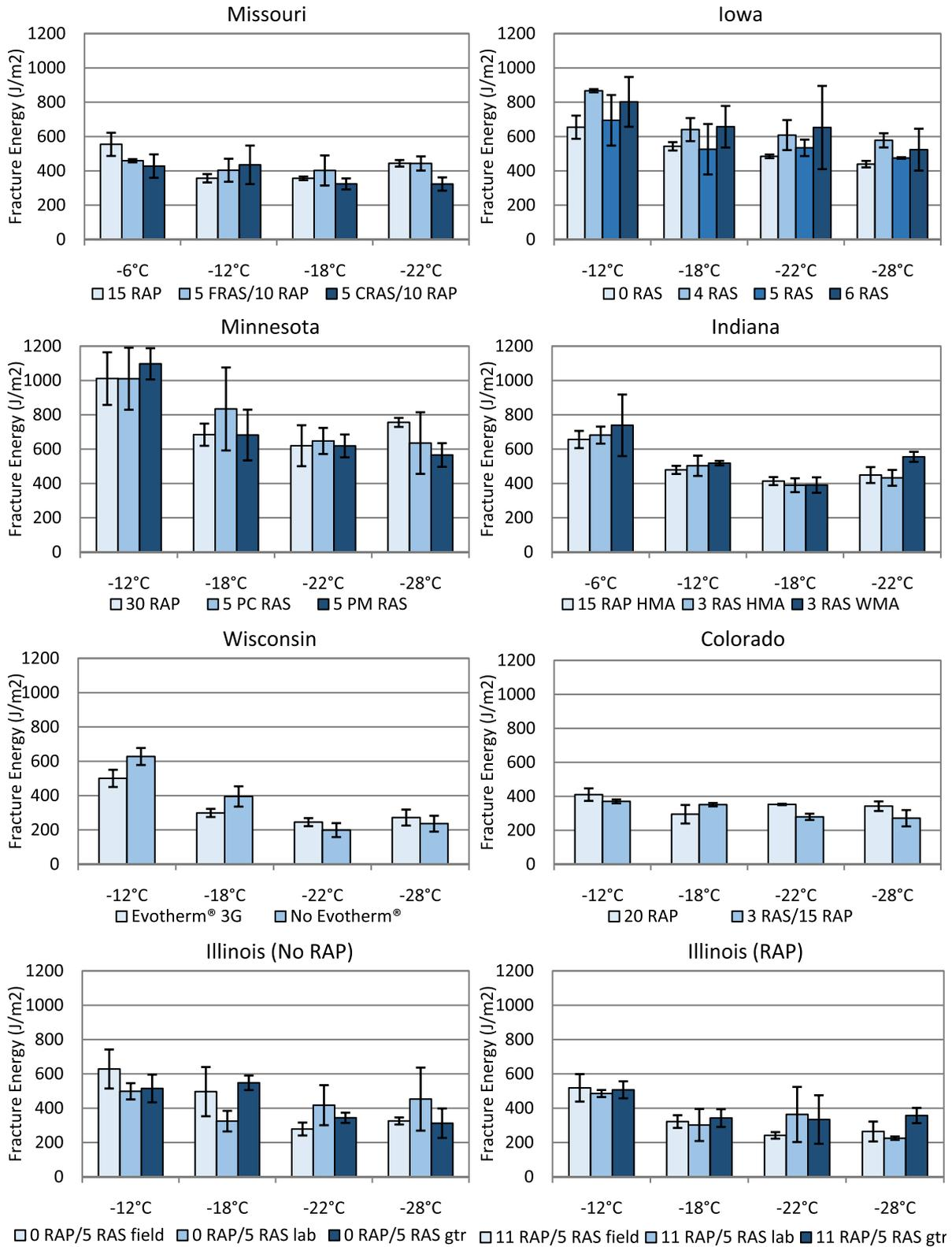
Fig. 9. Fracture energy ( $G_f$ ) of mixes from each state.
