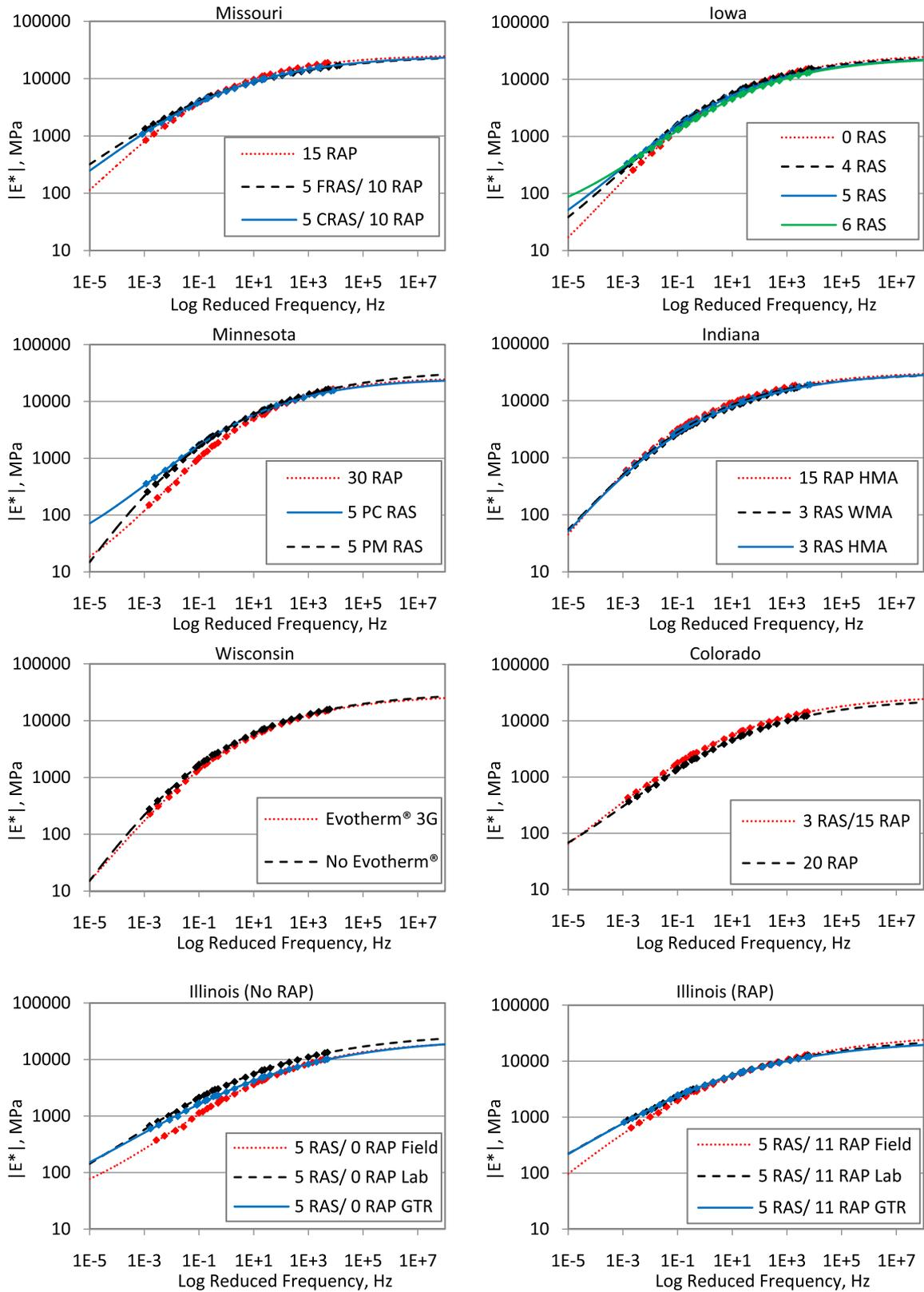
Fig. 6. Dynamic modulus master curves.
