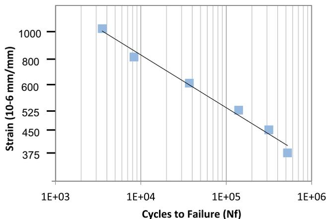
Fig. 1. Sample fatigue curve.
