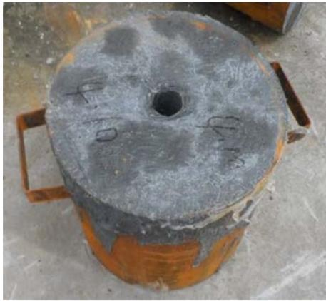
Fig. 2. Concrete target for different depth explosion (The cylindrical hole in the middle of the target is used for placing explosive).
