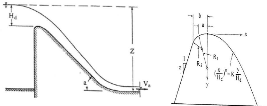
**Fig. 1:** Ogee spillway.
