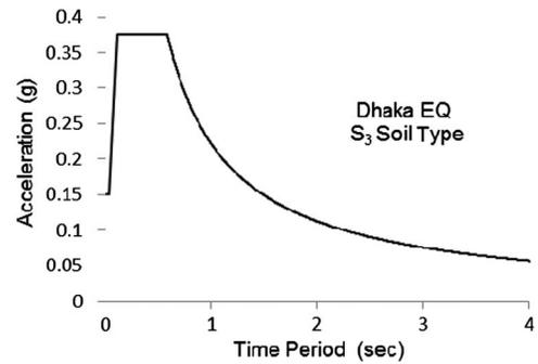
Fig. 7. Acceleration response spectrum for S3 soil for Dhaka
