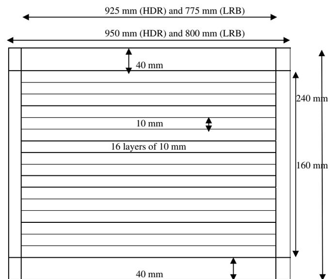
**Fig. 4.** High damping rubber bearing and lead rubber bearing dimensions
