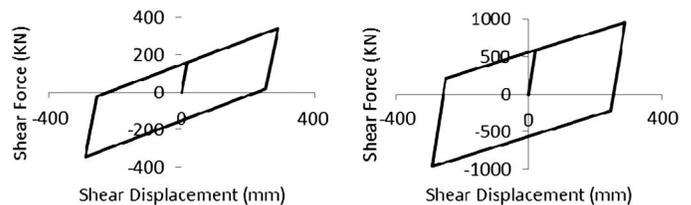
**Fig. 3.** Hysteresis of isolator LRB (left) & HDRB (right)
