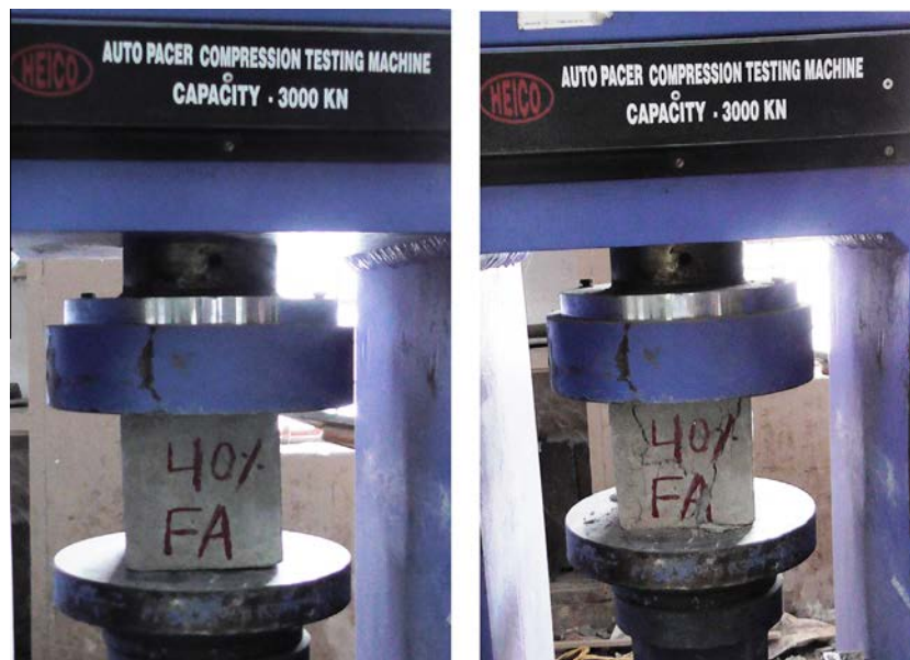
Fig. 5. Compression test (before and after test).
