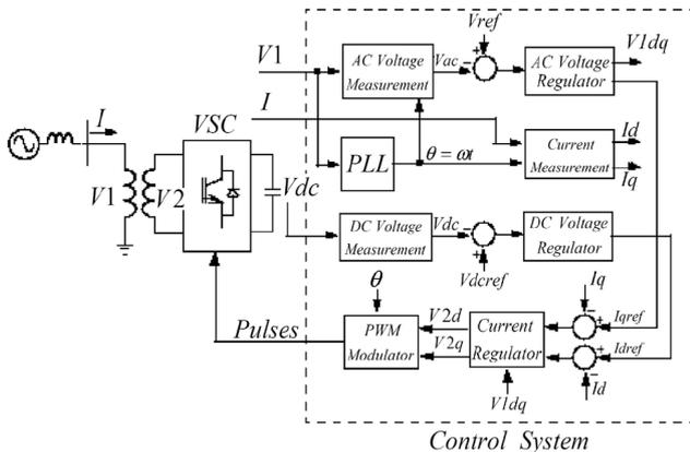
Figure 4. Control system block diagram of STATCOM
