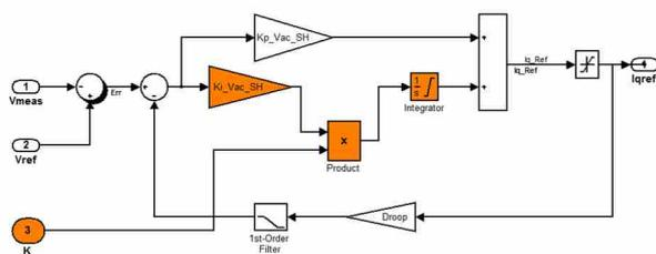
Figure 5. STATCOM voltage regulator with changes
