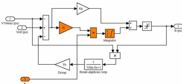
Figure 14. SVC voltage regulator with changes in order to select the optimal value of  $K$
