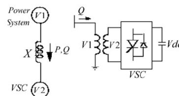
Figure 3. Operating principle of the STATCOM
