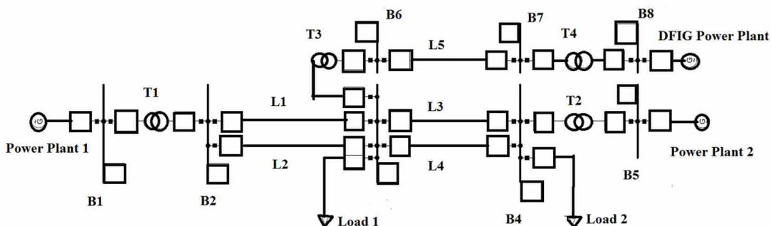
Figure 7. The single line diagram of the studied power system
