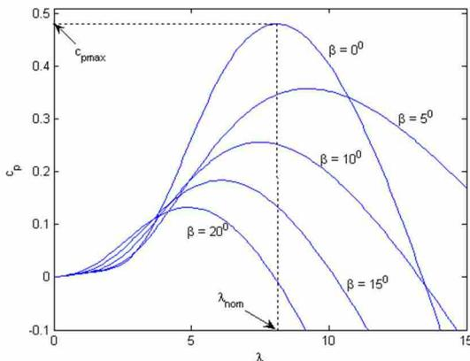
Figure 1. The  $C_p-\lambda$  characteristics for different values of the pitch angle  $\beta$
