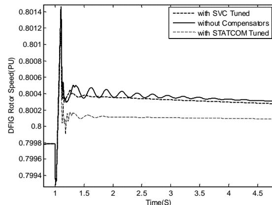
Figure 17. DFIG rotor speed with SVC and STATCOM tuned
