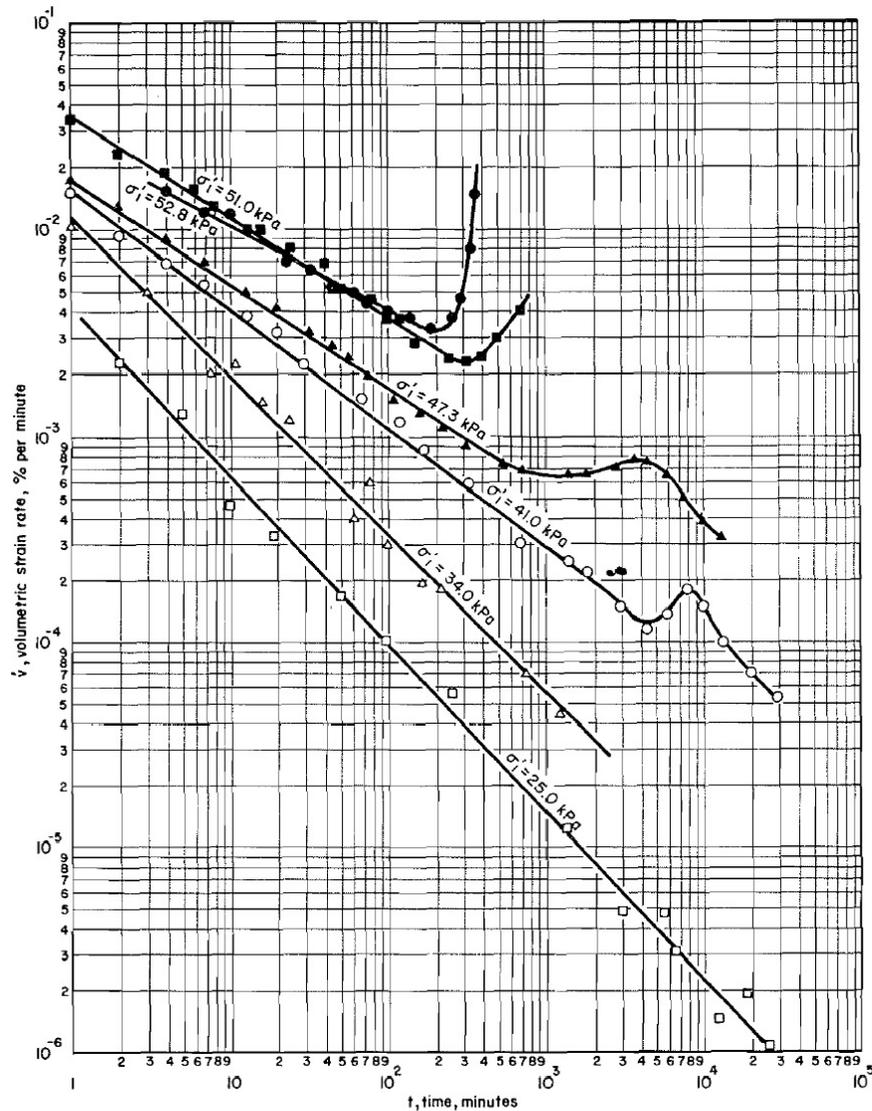
FIG. 3. Volumetric strain rate - time relationship for drained tests at  $\sigma'_s = 16.5$  kPa performed along line 3 (Fig. 1).
