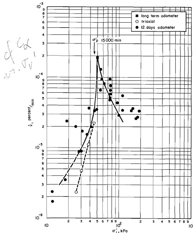
FIG. 10. Variations of the volumetric strain rate with  $\sigma_v'$  at  $t = 15\,000$  min.
