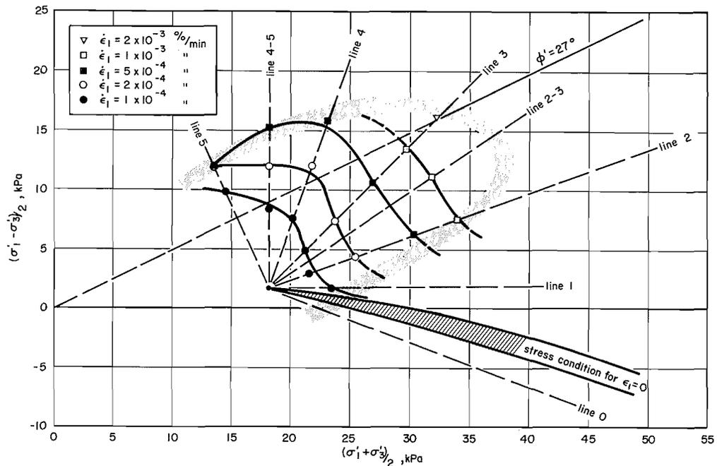
FIG. 16. Lines of equal axial strain rate at  $t = 100$  min in the stress space for drained tests.
