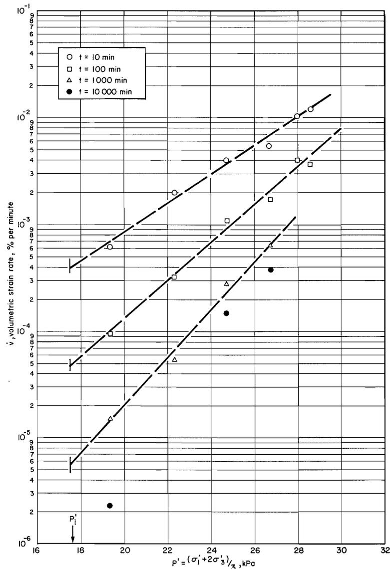
FIG. 4 Volumetric strain rate vs. mean normal effective stress in drained tests at  $\sigma'_3 = 16.5$  kPa performed along line 3 (Fig. 1).
