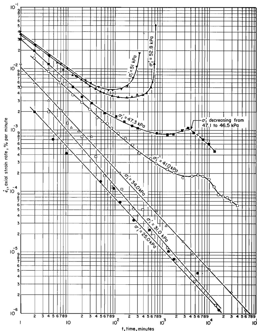
FIG. 12. Axial strain rate – time relationship for drained tests at  $\sigma'_v = 16.5$  kPa performed along line 3 (Fig. 1).
