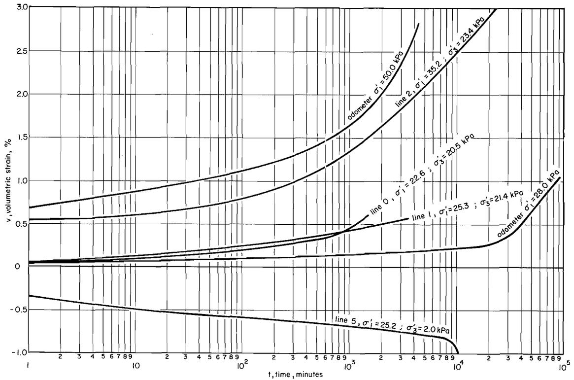
FIG. 5. Volumetric strain - time relationship for drained tests under various stress conditions.
