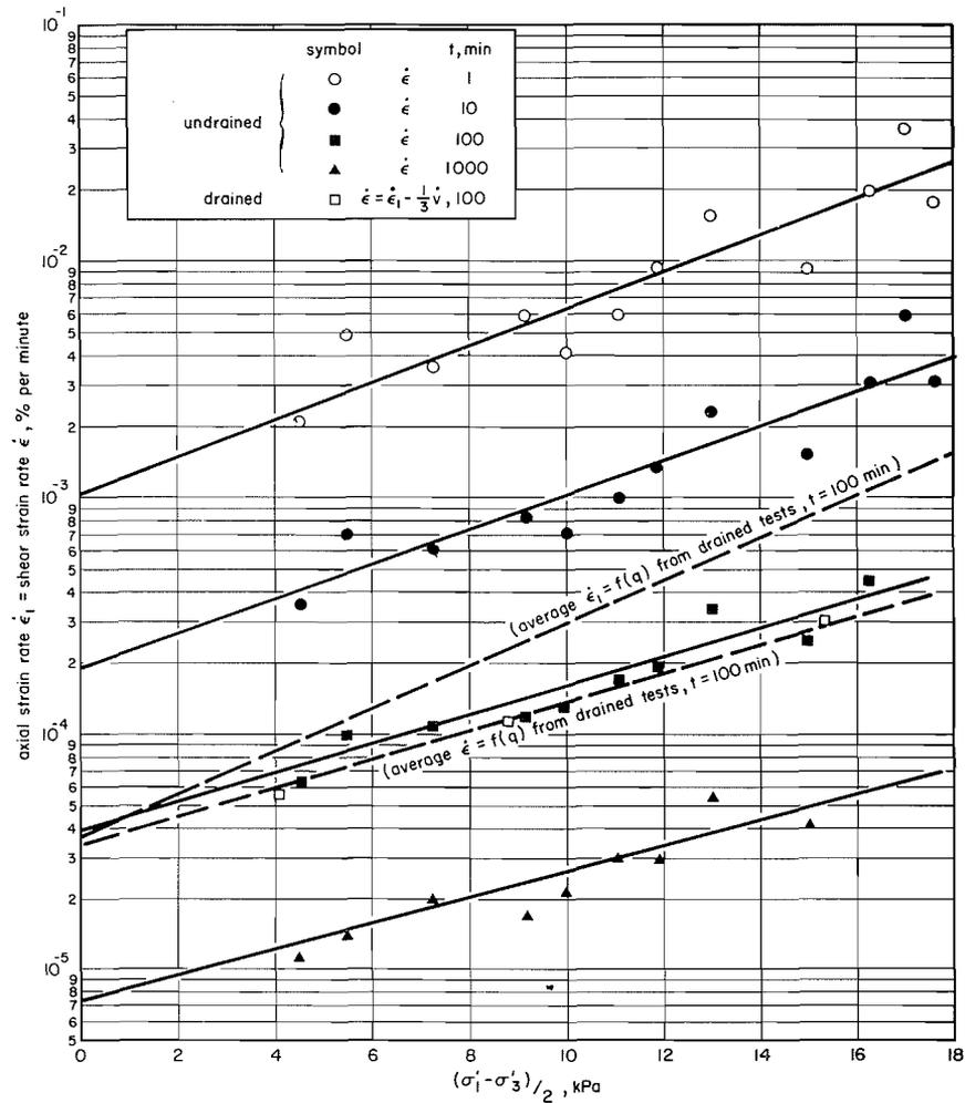
FIG. 18. Shear strain rate vs. shear stress for undrained and drained tests at  $\sigma'_{30} = 16.5$  kPa.
