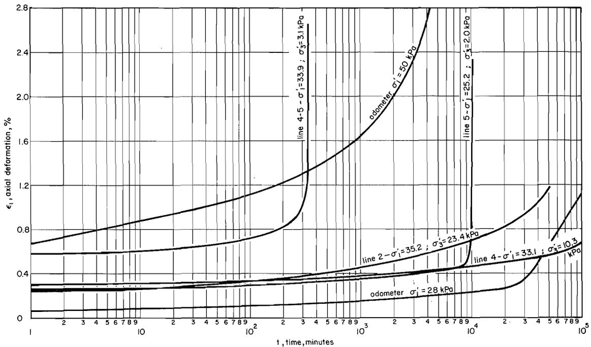
FIG. 14. Axial strain - time relationship for drained tests under various stress conditions.
