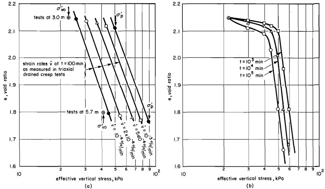
FIG. 9. Lines of equal volumetric strain rate and equal duration of loading in the  $e - \log \sigma_v'$  plane for drained tests.
