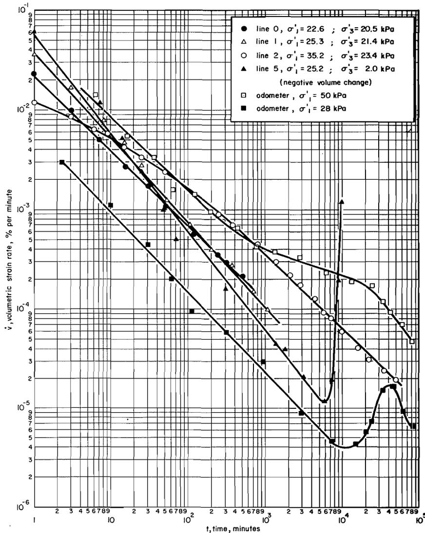
FIG. 6. Volumetric strain rate – time relationship for drained tests under various stress conditions.
