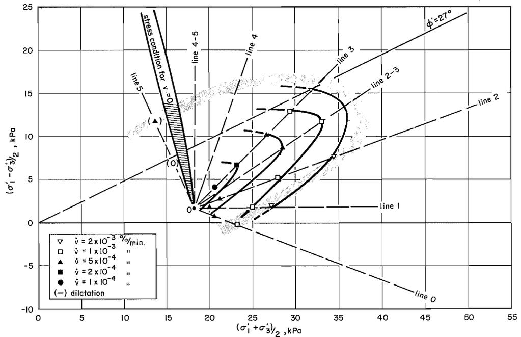
FIG. 8. Lines of equal volumetric strain rate at  $t = 100$  min in the stress space for drained tests.
