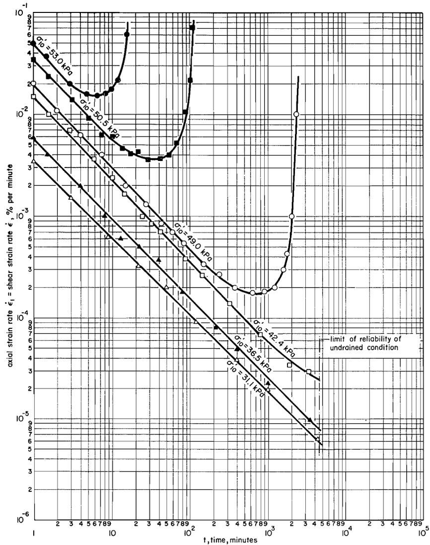
FIG. 17. Shear strain rate - time relationship for undrained tests at  $\sigma_{30}' = 16.5$  kPa.
