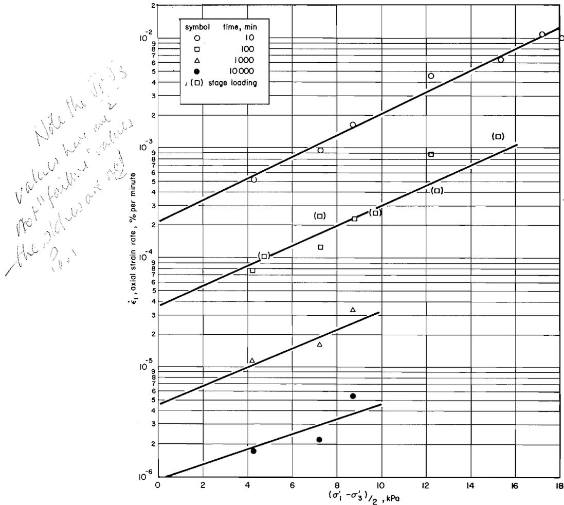
FIG. 13. Axial strain rate vs. shear stress for drained tests at  $\sigma'_3 = 16.5$  kPa performed along line 3 (Fig. 1).
