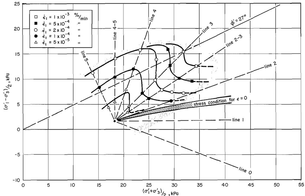
Fig. 19. Lines of equal shear strain rates at  $t = 100$  min in the stress space for drained and undrained tests.
