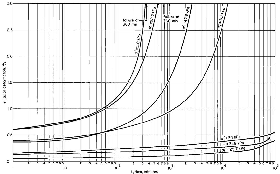
FIG. 11. Axial strain - time relationship for drained tests at  $\sigma'_s = 16.5$  kPa performed along line 3 (Fig. 1).
