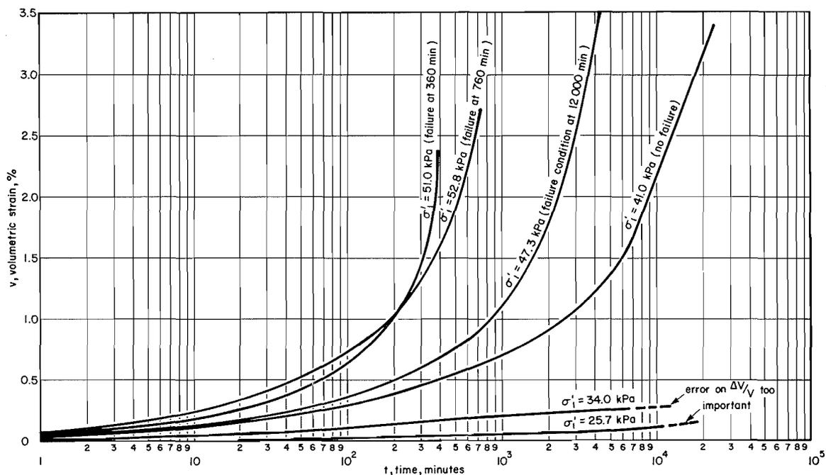
FIG. 2. Volumetric strain - time relationship for drained tests at  $\sigma_3' = 16.5$  kPa performed along line 3 (Fig. 1).
