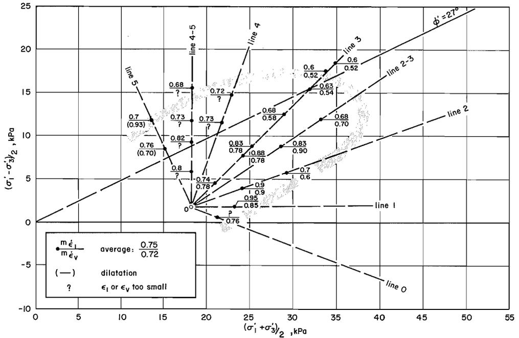
FIG. 7. Variations of the creep parameter  $m$  for volumetric and axial strains with the stress condition.
