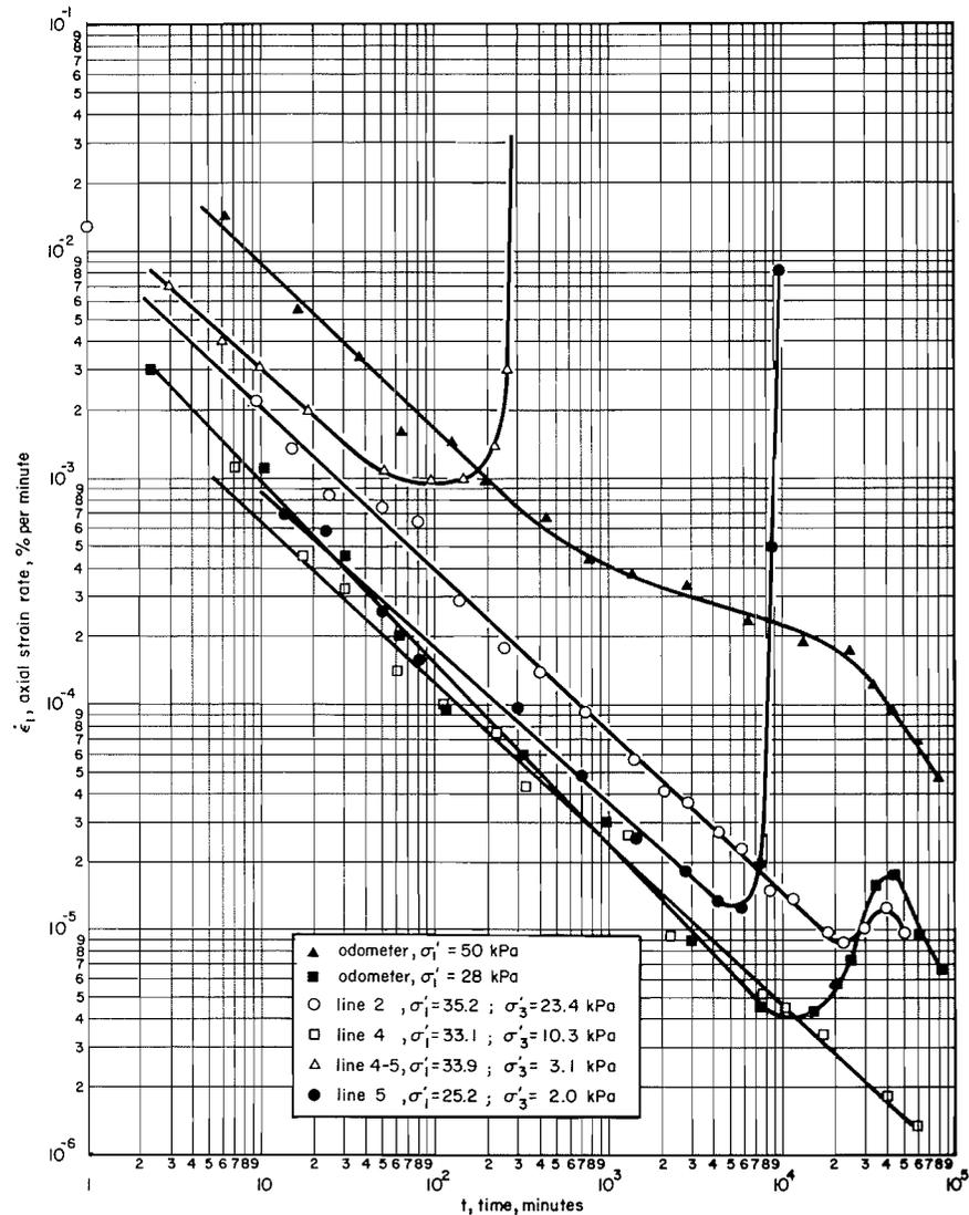
FIG. 15. Axial strain rate – time relationship for drained tests under various stress conditions.
