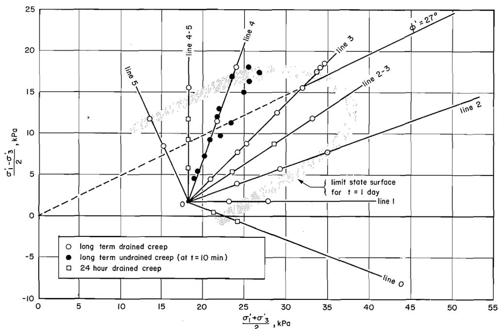
FIG. 1. Stress conditions for drained and undrained creep tests.
