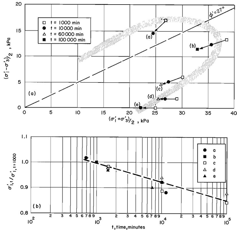
FIG. 20. Displacement of the limit state surface with time.
