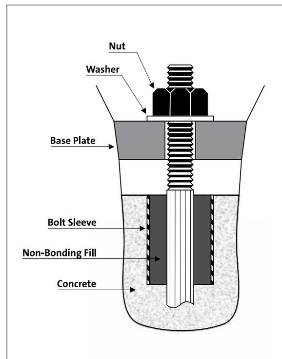
*Figure 5. Anchor Bolt and Pipe Sleeve Detail*
