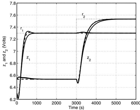
Fig. 6. Transient responses of the lower tank levels (solid line), reference model outputs (dashed line), and set-point signals (dotted) for the 4 polytope vertices.
