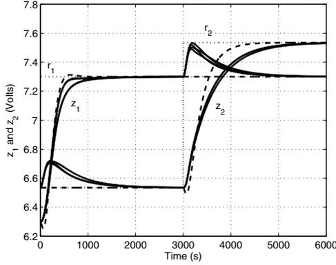
Fig. 5. Transient responses of the lower tank levels (solid line), reference model outputs (dashed line), and set-point signals (dotted) for the 4 polytope vertices.
