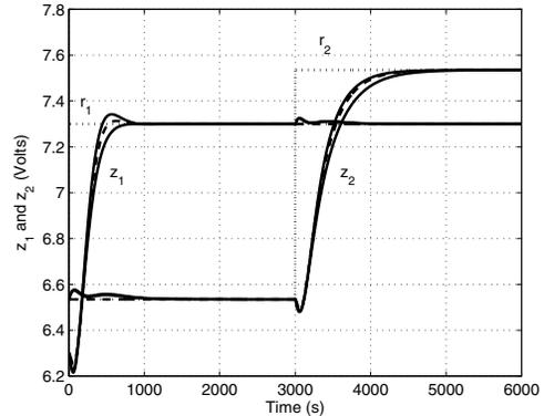
Fig. 3. Transient responses of the lower tank levels (solid line), reference model outputs (dashed line), and set-point signals (dotted) for the 4 polytope vertices.
