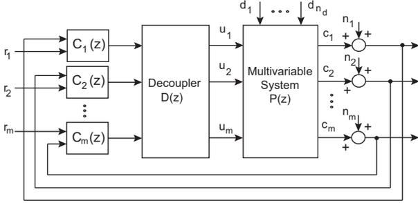
Fig. 1. Decoupling Control.
