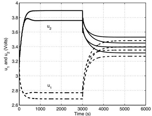
Fig. 4. Transient responses of the pump voltages  $u_1$  (dashed line) and  $u_2$  (solid line) for the 4 polytope vertices.
