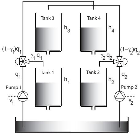
Fig. 2. Quadruple-tank process.
