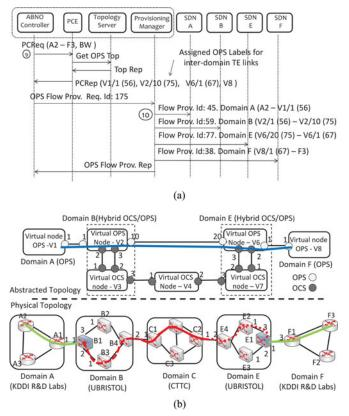
Fig. 7. OPS flow provisioning. (a) Workflow for an OPS flow provisioning (A2-F3). (b) Abstract and physical network view.
