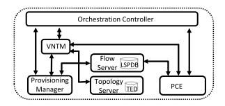
Fig. 1. ABNO-based orchestrator architecture.
