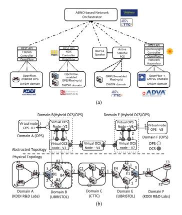
Fig. 4. Experimental network scenario. (a) International Testbed of the STRAUSS project. (b) Abstract and physical network view.
