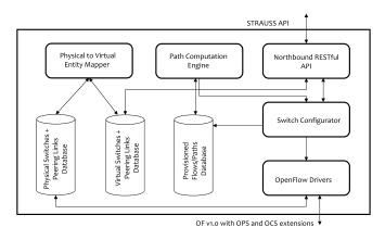
Fig. 5. OpenFlow controller for hybrid OPS-OCS domains.
