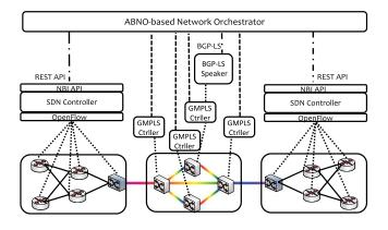
Fig. 2. ABNO-based network orchestrator with physical network topology and centralized path computation.
