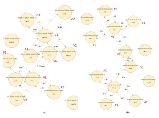
Fig. 8. Abstract OPS network topology seen by the ABNO-based orchestrator's PCE drawn as a directed graph. (a) Before the provisioning of the OPS Link between V2 and V6. (b) After the provisioning of the OPS Link between V2 and V6.
