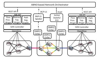
Fig. 3. ABNO-based network orchestrator with abstracted network topology and distributed path computation.
