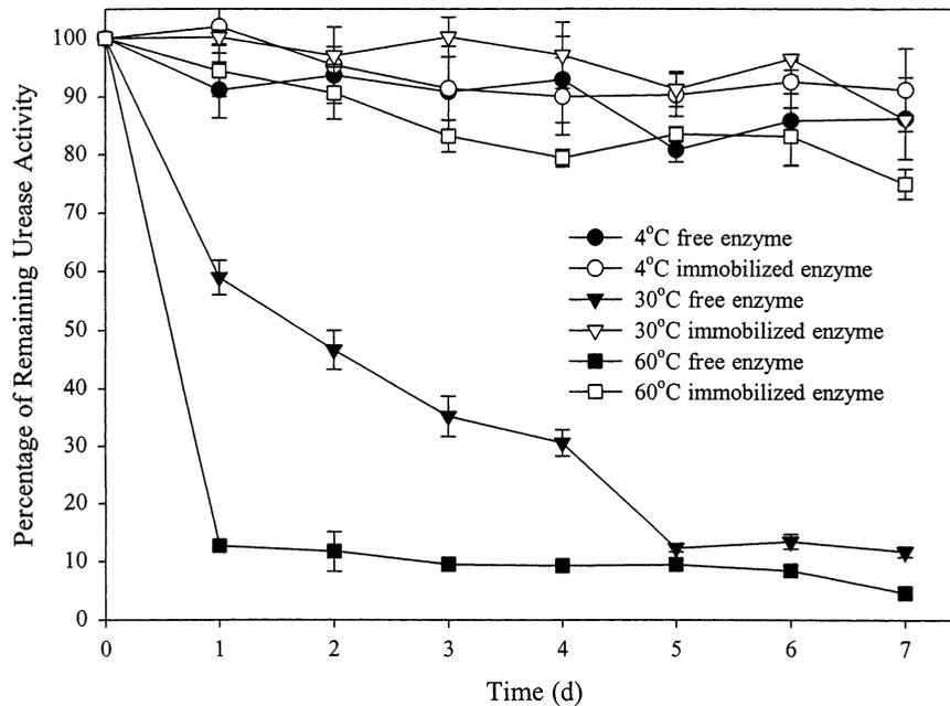
Fig. 6. Effects of temperature on the free and immobilized urease.
