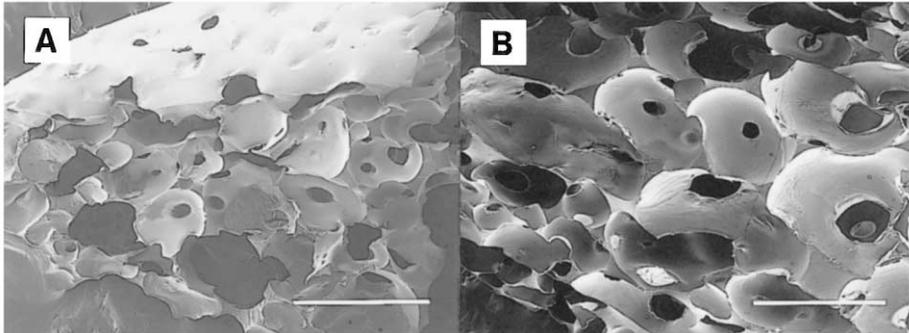
Fig. 3. Scanning electron micrographs of polyurethane foam showing porous matrices. (A) PU matrices close to the surface area (bar, 1 mm). (B) PU matrices toward the inside (bar, 1 mm).
