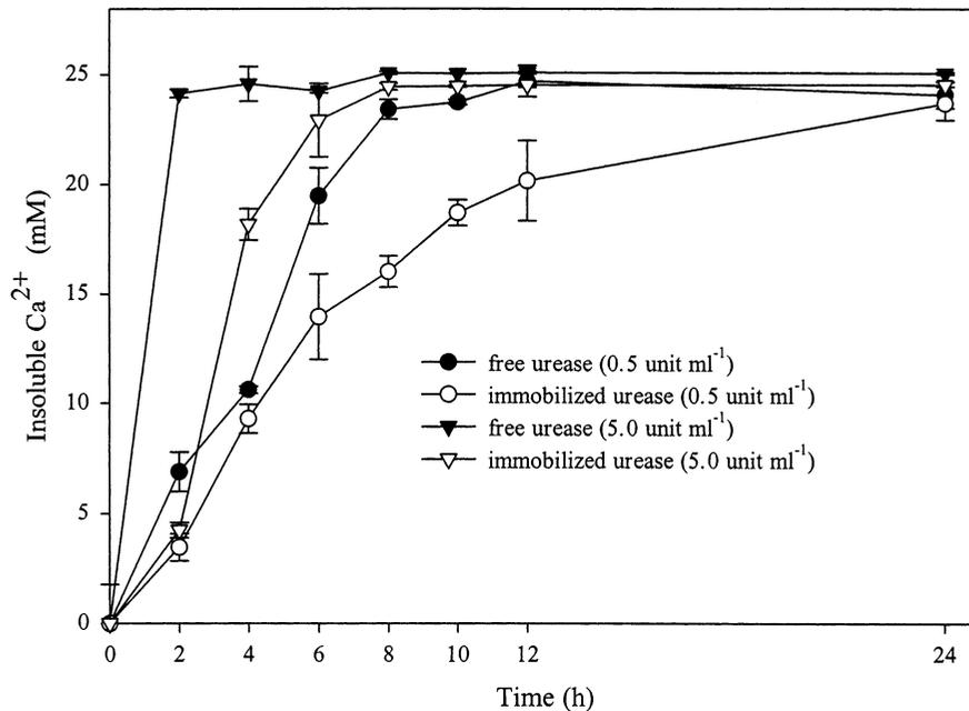
Fig. 4. Calcite precipitation induced by the free and immobilized urease.
