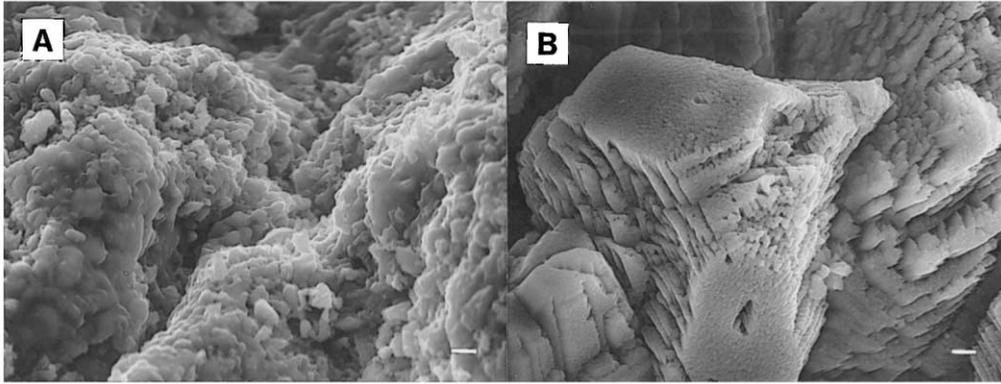
Fig. 5. Scanning electron micrographs of calcite precipitation induced by the PU-immobilized urease. (A) Calcite precipitation on the surface area of PU foam showing small and less organized crystals (bar, 1  $\mu\text{m}$ ). (B) Calcite precipitation within the matrices of PU foam showing typical and well organized crystals (bar, 1  $\mu\text{m}$ ).
