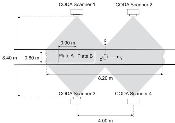
Fig. 1. Location of force plates and CODA scanners for kinetic data collection; the shaded area indicates the field of view of the CODA scanners.
