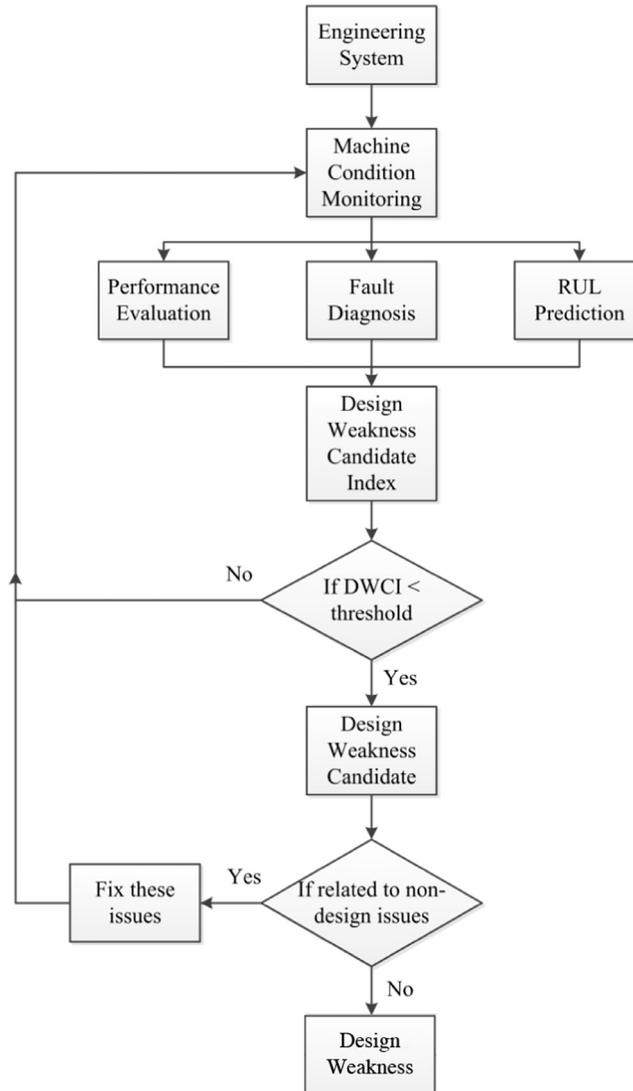
Fig. 4. Procedure of design weakness detection.
