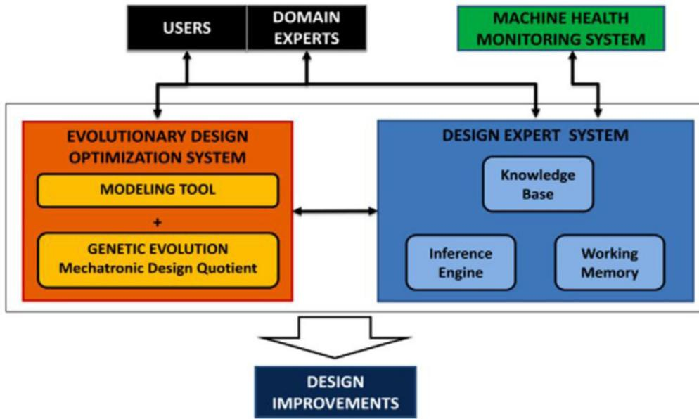
Fig. 1. System framework of design evolution with machine health monitoring system [16].
