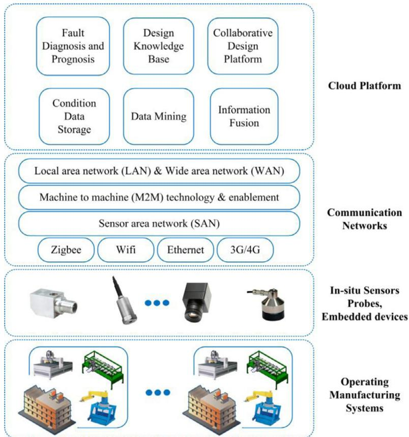
Fig. 3. Proposed scheme of condition monitoring through the IoT and CC.
