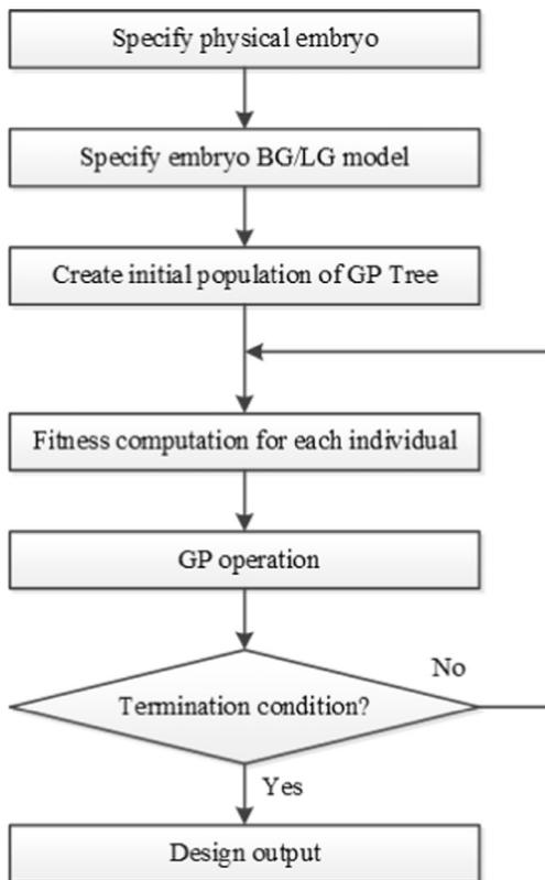
**Fig. 7.** Procedure of evolutionary design with GP.
