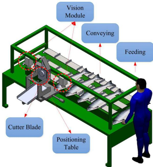
Fig. 5. Schematic diagram of the automated fish cutting system.
