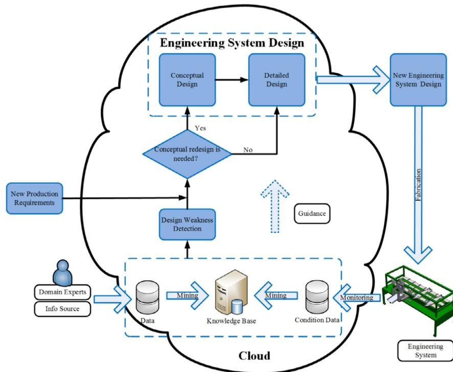
Fig. 2. Framework for closed-loop design evolution of an engineering system.
