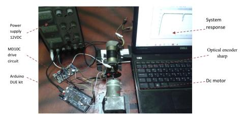
Figure 6 Real system of the DC motor speed control using Arduino DUE.
