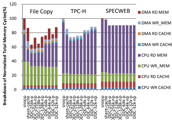
Figure 19 Breakdown of Normalized Total Memory Cycles with Write-Through Policy
