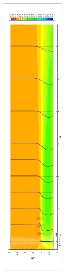
Figure 4: Contours of dimensionless axial velocity, plane  $x = 0, k - \omega$  model
