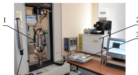
Fig. 2. View of measuring apparatus: 1 – testing machine MTS with sleeve-punch assembly, 2 – chamber for material seasoning, 3 – moisture analyser.
