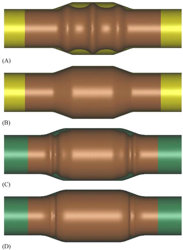
**Fig. 15 – Forming processes under 5.0 MPa internal pressure in the pre-forming stage. (A) After feeding pressure in the pre-forming stage; (B) after calibration pressure in the pre-forming stage; (C) after feeding pressure in the finishing stage; (D) after calibration pressure in the finishing stage.**
