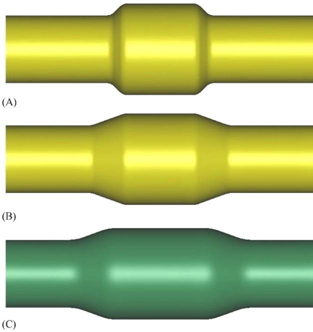
**Fig. 6 – Modeled die cavities used in simulation. (A) 45° pre-forming die cavity; (B) 25° pre-forming die cavity; (C) final die cavity.**
