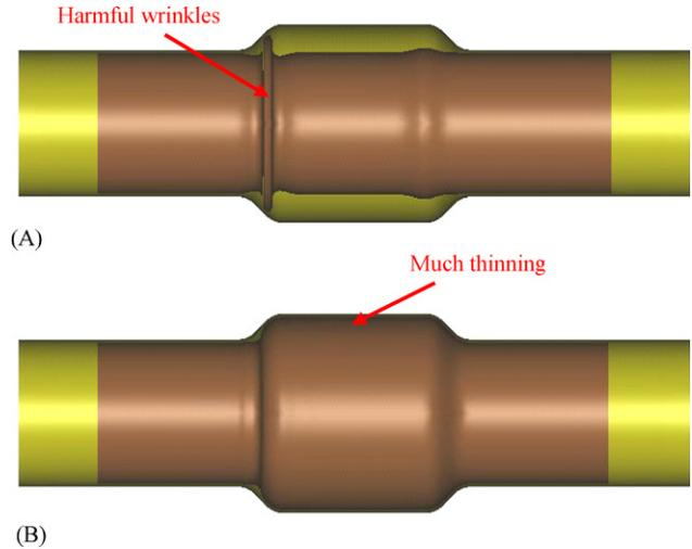
**Fig. 8 – Forming processes under 1.0 MPa feeding pressure in the pre-forming stage. (A) After the feeding pressure; (B) after the calibration pressure.**
