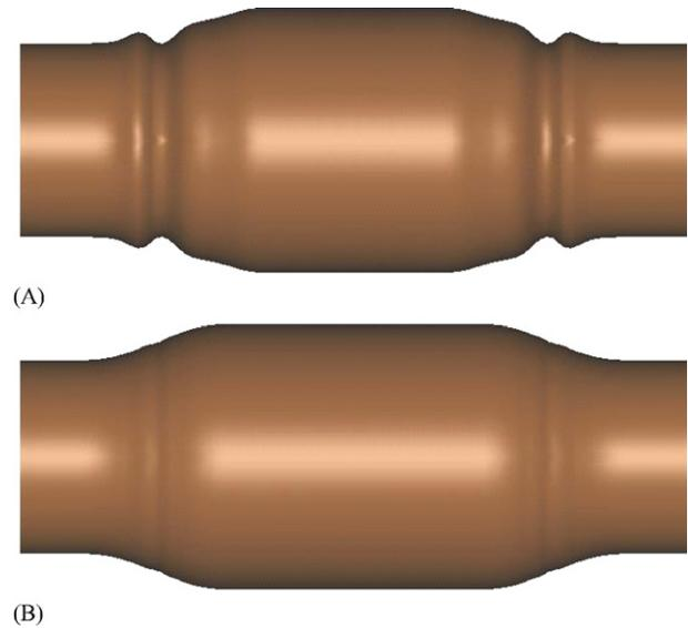
**Fig. 18 – Final part by shortening the punch strokes to 3.0 mm in the finishing stage. (A) After feeding pressure; (B) after calibration pressure.**
