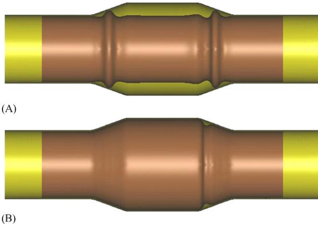
**Fig. 13 – Formed forming processes under 1.0 MPa internal pressure in the pre-forming stage. (A) After feeding pressure; (B) after calibration pressure.**
