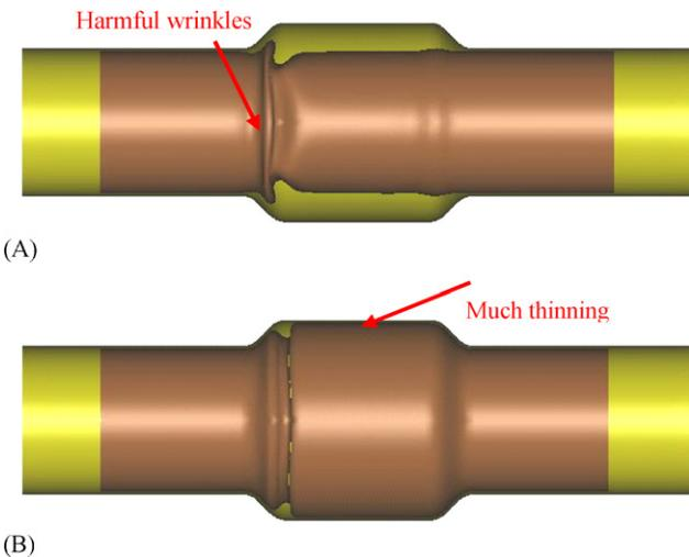
**Fig. 7 – Forming processes without feeding pressure in the pre-forming stage. (A) Without the feeding pressure; (B) after the calibration pressure.**
