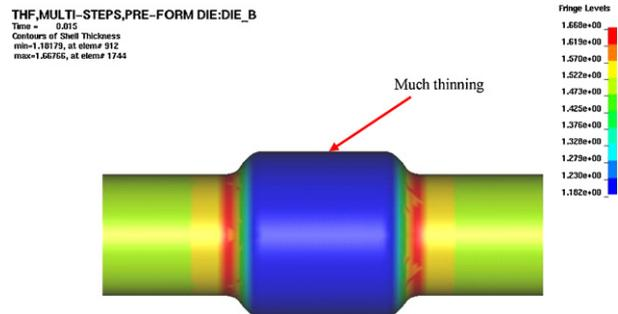
**Fig. 12 – Thickness distribution when using 7.0 MPa feeding pressure in the pre-forming stage.**
