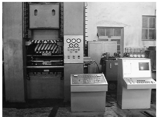
**Fig. 23 – Photograph of tube hydroforming equipment.**
