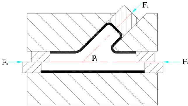
Fig. 1 – Description of tube hydroforming.
