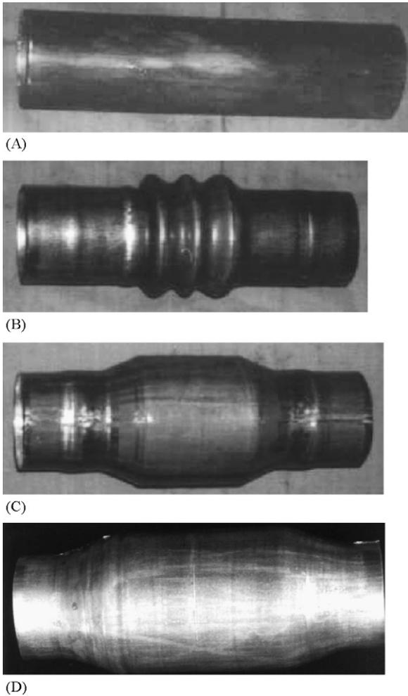
**Fig. 24 – Different forming stages. (A) Tube blank; (B) useful wrinkles in pre-forming stage; (C) pre-formed part; (D) finally formed part.**
