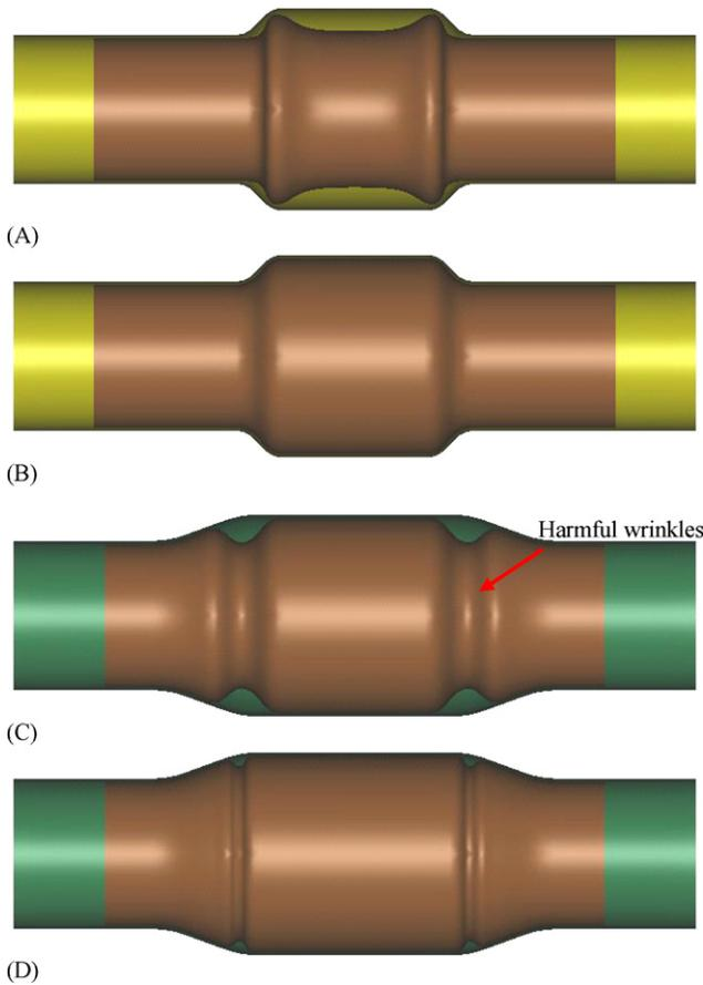
**Fig. 10 – Forming processes under 5.0 MPa feeding pressure in the pre-forming stage. (A) After feeding pressure in the pre-forming stage; (B) after calibration pressure in the pre-forming stage; (C) after feeding pressure in the calibration stage; (D) after calibration pressure in the calibration stage.**
