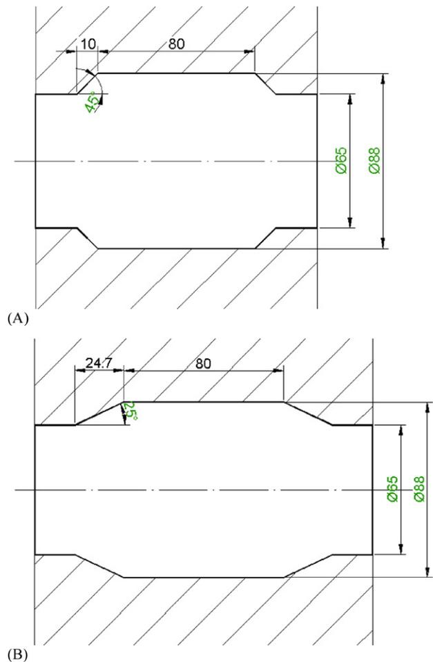
**Fig. 5 – Pre-forming die cavities used. (A) 45° pre-forming die cavity; (B) 25° pre-forming die cavity.**
