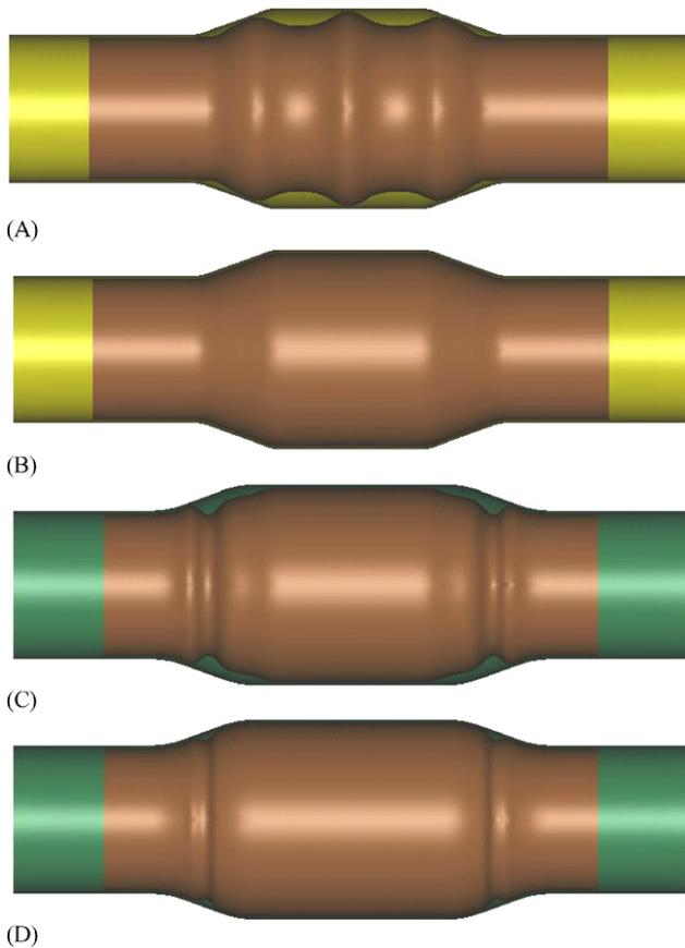
**Fig. 16 – Forming processes under 6.0 MPa internal pressure in the pre-forming stage. (A) After feeding pressure in the pre-forming stage; (B) after calibration pressure in the pre-forming stage; (C) after feeding pressure in the finishing stage; (D) after calibration pressure in the finishing stage.**
