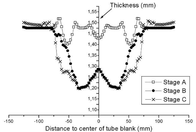
**Fig. 19 – Wall thickness distributions in different stages under feeding pressure of 3.0 MPa in the pre-forming stage.**
