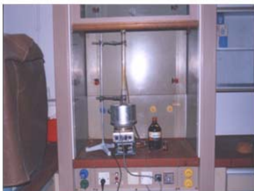
Figure 1. Heating acetonitril, bromohexadecane and trimethyl amine mixture under vacuum air condition.
