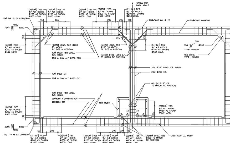
Figure 4 Typical Reinforcing Details of Side-by-Side Box
