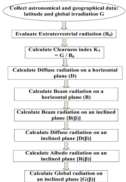
Fig. 5. Algorithm for calculation of global radiation on tilted PV panels.
