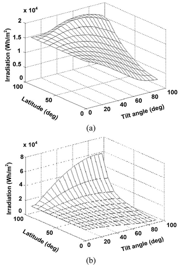
Fig. 7. Irradiation as a function of tilt angle and latitude of northern hemisphere for from (a) April to June, and (b) July through September.
