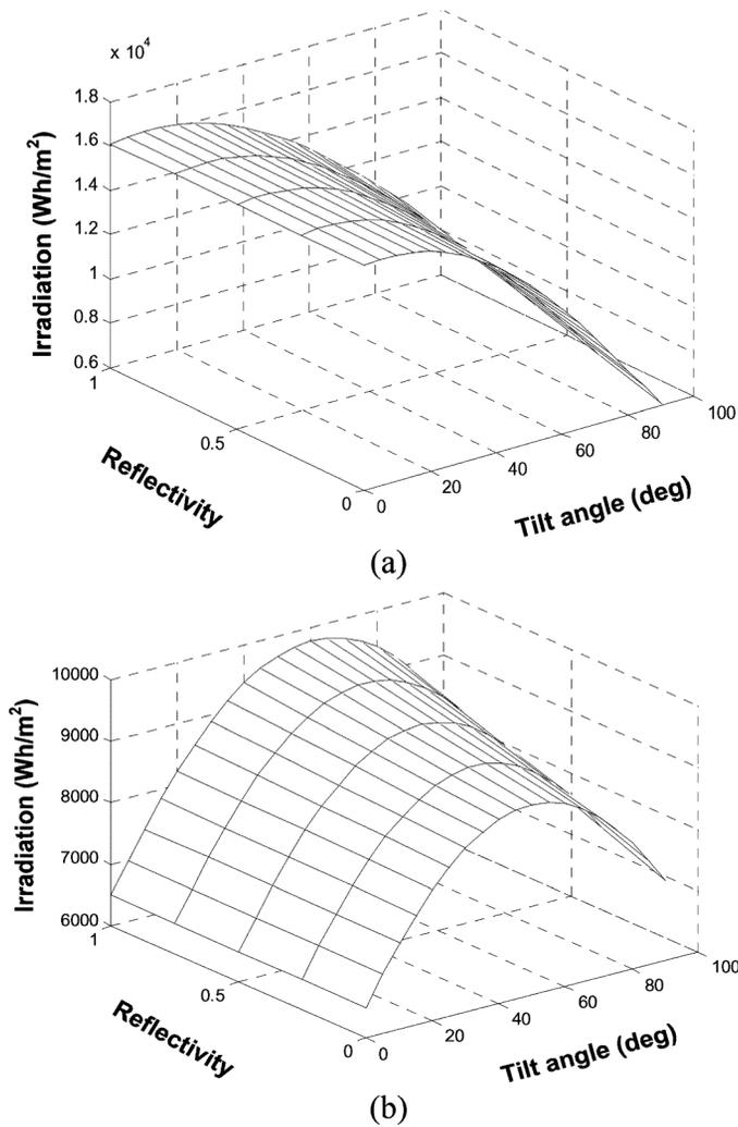
Fig. 6. Irradiation as a function of tilt angle and reflectivity for Columbus, Ohio from (a) April to June, and (b) October through December.
