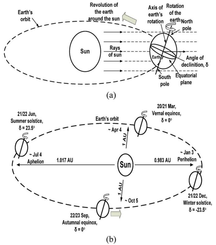
Fig. 2. Orbit of the earth around the sun over a year (a) defining the angles (b) detailing the orbit of the earth [8].
