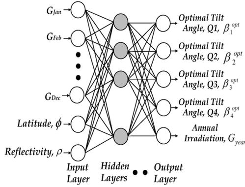
Fig. 8. Structure of NN for estimation of optimal tilt angle.
