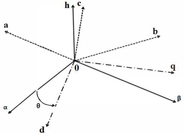
Figure 2. Two-axis ( $h\alpha\beta$  and  $hdq$  frames) and three-axis ( $abc$  frame) references representation
