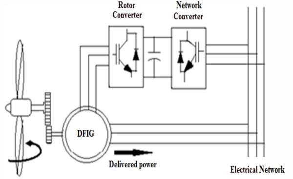
Figure 1. Wind energy conversion chain system based on DFIG
