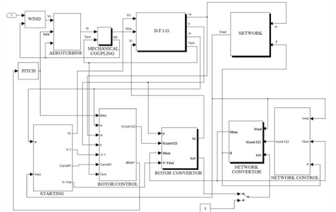
Figure 3. Simulink model of the wind energy conversion chain system based on DFIG
