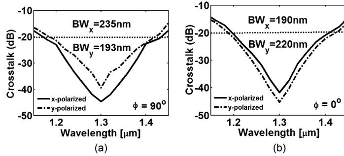
Fig. 8. Wavelength dependent crosstalk of the proposed MUX/DEMUX at core  $\beta$  around the operating wavelength  $\lambda = 1.3\text{ }\mu\text{m}$  at (a)  $\varphi = 90^\circ$  and (b)  $\varphi = 0^\circ$ .
