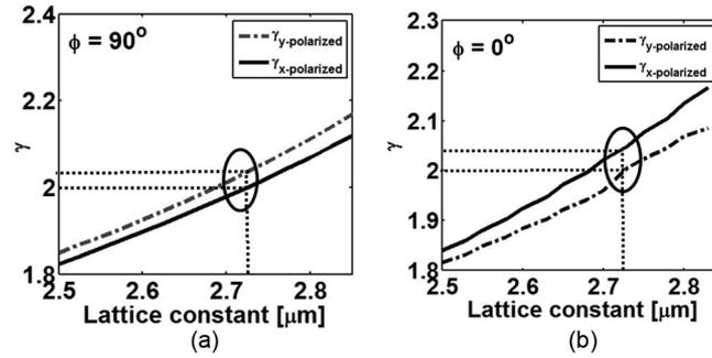
Fig. 6. Variation of the ratio between the coupling lengths at wavelengths of 1.3  $\mu\text{m}$  and 1.55  $\mu\text{m}$  for x-polarized and y-polarized modes with the hole pitch at (a)  $\varphi = 90^\circ$  and (b)  $\varphi = 0^\circ$ .
