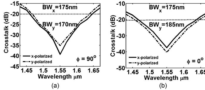
Fig. 9. Wavelength dependent crosstalk of the proposed MUX/DEMUX at core  $B$  around the operating wavelength  $\lambda = 1.55\text{ }\mu\text{m}$  at (a)  $\varphi = 90^\circ$  and (b)  $\varphi = 0^\circ$ .
