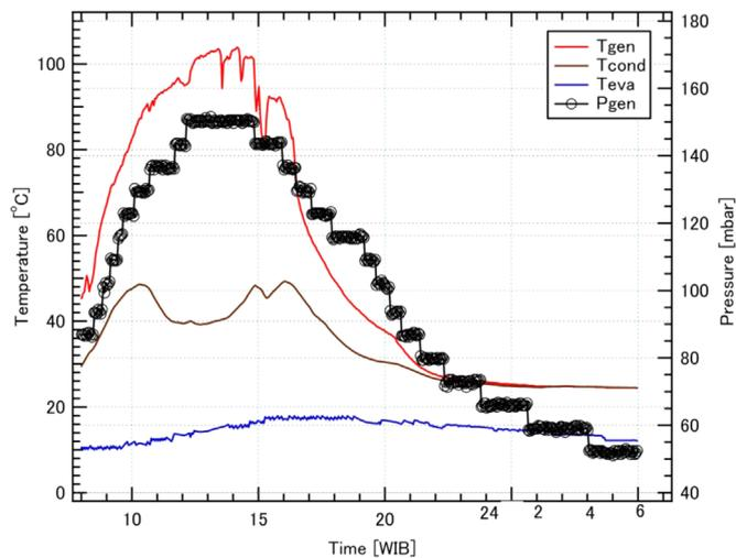
**Fig. 6.** Temperature and pressure history for 75AA case. (For interpretation of the references to color in this figure, the reader is referred to the web version of this article.)
