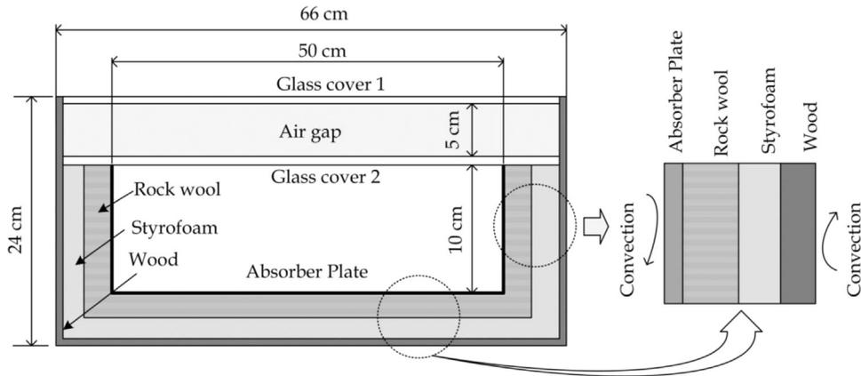
Fig. 2. Solar collector and its main dimensions.
