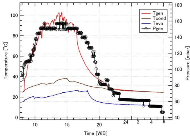
**Fig. 5.** Temperature and pressure history for 100AA case. (For interpretation of the references to color in this figure, the reader is referred to the web version of this article.)
