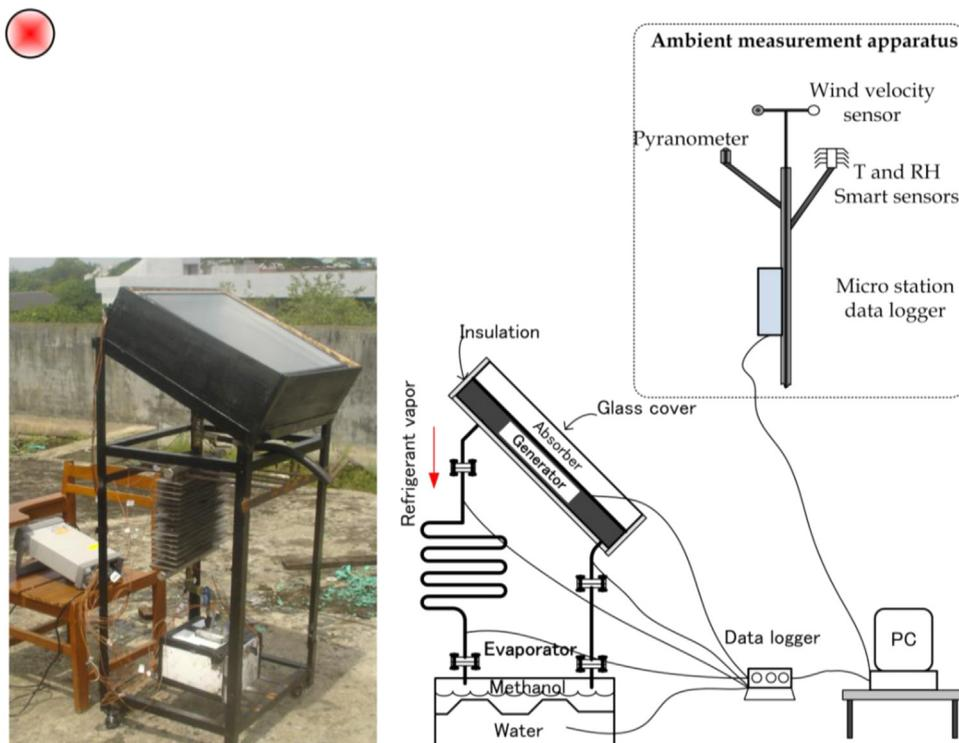
**Fig. 3.** Experimental apparatus and data acquisition system. (For interpretation of the references to color in this figure, the reader is referred to the web version of this article.)
