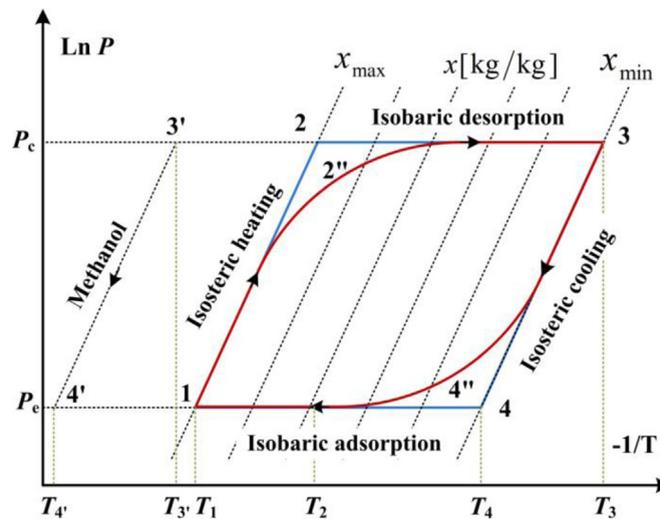
Fig. 1. The Clapeyron diagram of the adsorption refrigeration cycle.
