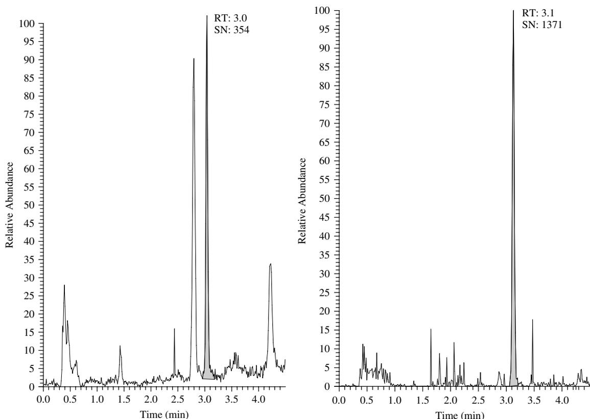
**Figure 16.** Mass selected liquid chromatogram of norverapamil in urine. The chromatogram on the left is without FAIMS selectivity and the one on the right shows significant improvement of signal-to-noise when FAIMS is selected for norverapamil. Shaded peak is that of norverapamil. (From Kapron J, Barnett DA. Thermo Electron Corporation Application Note: 362, 2006.) Copyright (2006) with permission from Thermo Fisher.
