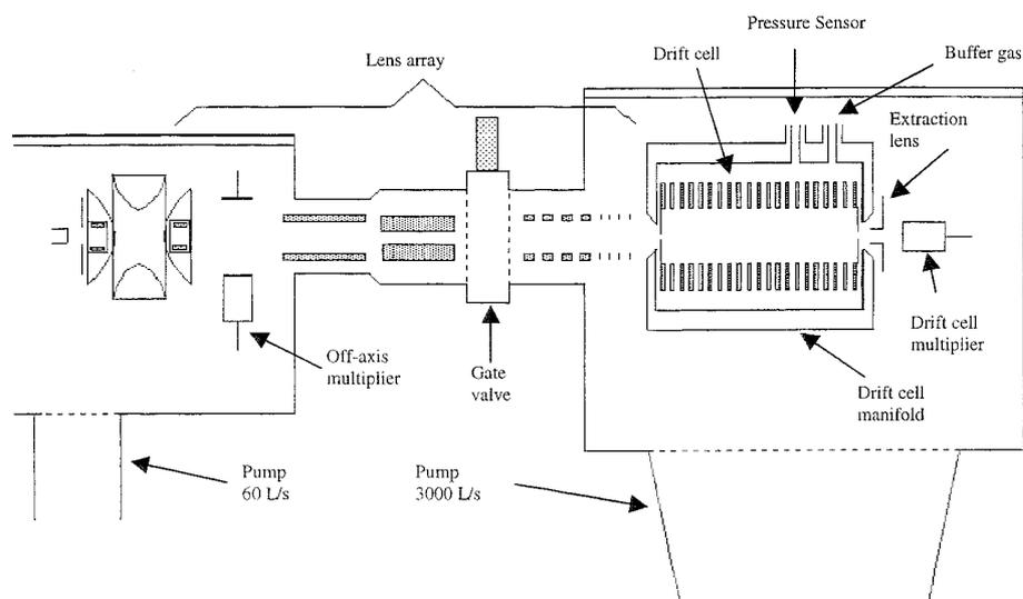
**Figure 19.** Schematic diagram of a tandem ion trap/ion mobility spectrometer. Reprinted from Creaser CS, Benyazzar M, Griffiths JR, Stygall JW. A tandem ion trap/ion mobility spectrometer. *Analytical Chemistry* 2000; **72**: 2724–2729. Copyright (2000) American Chemical Society.
