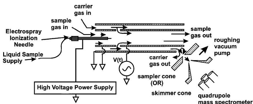
**Figure 14.** Schematic of an ESI-DMS instrument interfaced to a quadrupole mass spectrometer Reprinted from Guevremont R, Purves RW. High-field asymmetric-waveform ion mobility spectrometry–mass spectrometry: an investigation of leucine enkephalin ions produced by electrospray ionization. *Journal of the American Society for Mass Spectrometry* 1999; **10**: 492–501. Copyright (1999) with permission from Elsevier.
