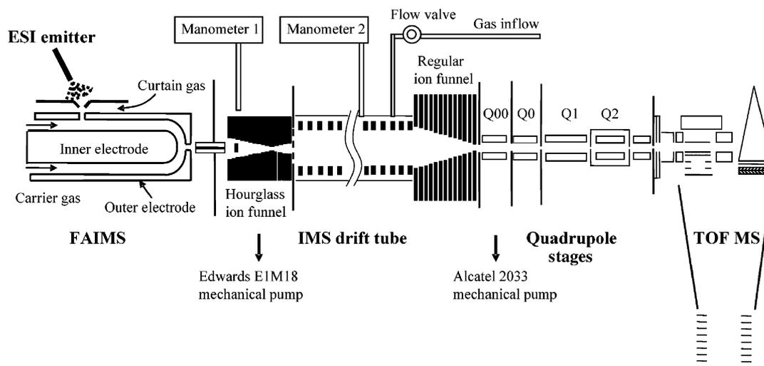
**Figure 9.** DMS-IMS-TOFMS design using an ion funnel as the interface between the ambient-pressure DMS and the reduced pressure IMS. Reprinted from Tang K, Li F, Shvartsburg AA, Strittmatter EF, Smith RD. Two-dimensional gas-phase separations coupled to mass spectrometry for analysis of complex mixtures. *Analytical Chemistry* 2005; **77**: 6381–6388. Copyright (2005) American Chemical Society.
