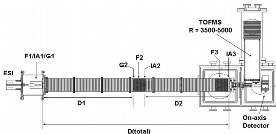
**Figure 4.** Schematic of an IMS-IMS-TOF Reprinted from Merenbloom SI, Bohrer BC, Koeniger SL, Clemmer DE. 'Assessing the peak capacity of IMS-IMS separations of tryptic peptide ions in He at 300K', *Analytical Chemistry* 2007; **79**: 515–522. Copyright (2007) American Chemical Society.
