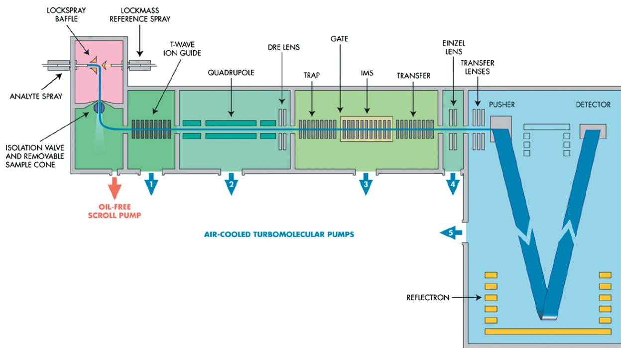
**Figure 5.** Synapt HDMS system reprinted from Pringle SD, Giles K, Wildgoose JL, Williams JP, Slade SE, Thalassinos K, Bateman RH, Bowers MT, Scrivens JH. An investigation of the mobility separation of some peptide and protein ions using a new hybrid quadrupole/traveling wave IMS/TOF instrument. *International Journal of Mass Spectrometry* 2007; **261**: 1–12. Copyright (2007) with permission from Elsevier.
