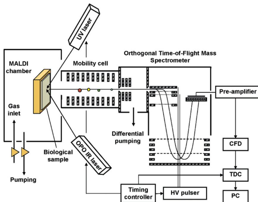
**Figure 7.** Schematic of IR and UV-MALDI-IM-oTOF-MS. Reprinted from Woods AS, Ugarov M, Jackson SN, *et al.* “IR-MALDI-LDI combined with ion mobility orthogonal time-of-flight mass spectrometry”. *Journal of Proteome Research* 2006; 5: 1484–1487. Copyright (2006) with permission from American Chemical Society.
