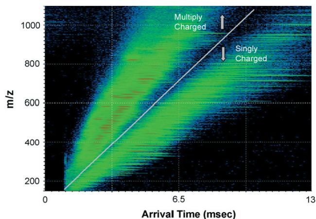
**Figure 6.** A 2D plot of ion-arrival time *versus*  $m/z$  for a protein digest mixture obtained using TWIMS. Reprinted from Pringle SD, Giles K, Wildgoose JL, Williams JP, Slade SE, Thalassinos K, Bateman RH, Bowers MT, Scrivens JH. An investigation of the mobility separation of some peptide and protein ions using a new hybrid quadrupole/traveling wave IMS/TOF instrument. *International Journal of Mass Spectrometry* 2007; **261**: 1–12. Copyright (2007) with permission from Elsevier.
