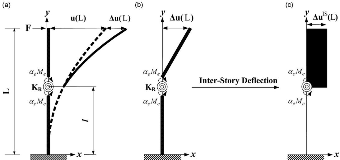
Fig. 2. (a) Deflection due to damage and applied force of a damaged cantilever beam, (b) damage-induced deflection and (c) damage-induced inter-storey deflection.
