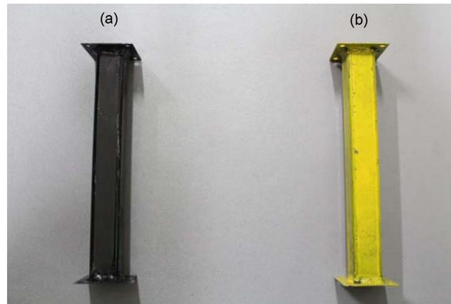
Fig. 14. (a) Intact column and (b) damaged column.
