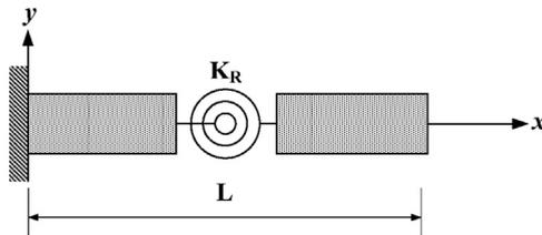
Fig. 1. Structure with torsional spring representation of damage.
