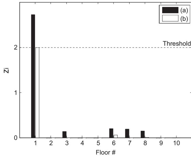
Fig. 23. Investigation of the damage location(s) by the damage index approach (a) DC1 and (b) DC2.
