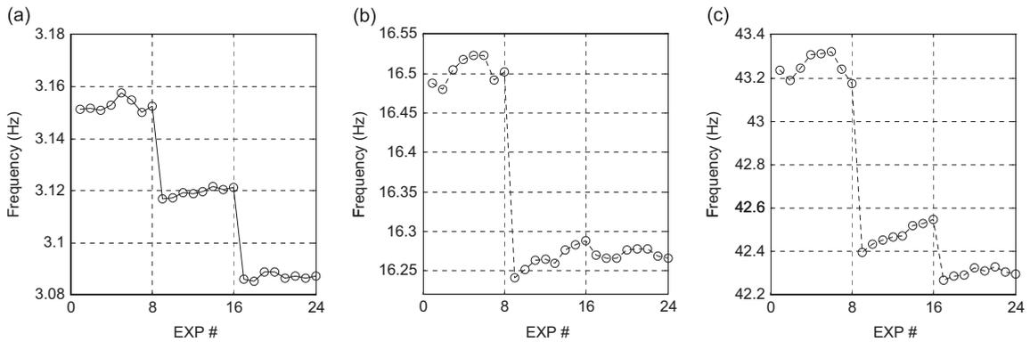
Fig. 16. Evolutions of the natural frequencies for (a) the first mode, (b) the second mode and (c) the third mode.
