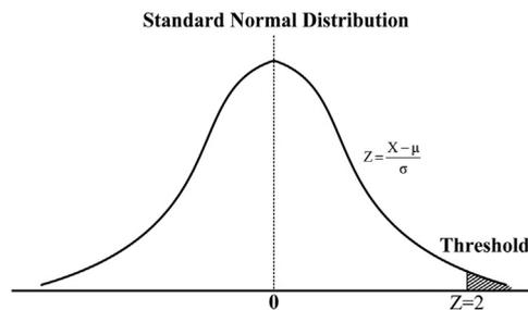
Fig. 5. Outlier analysis based on standard normal distribution.
