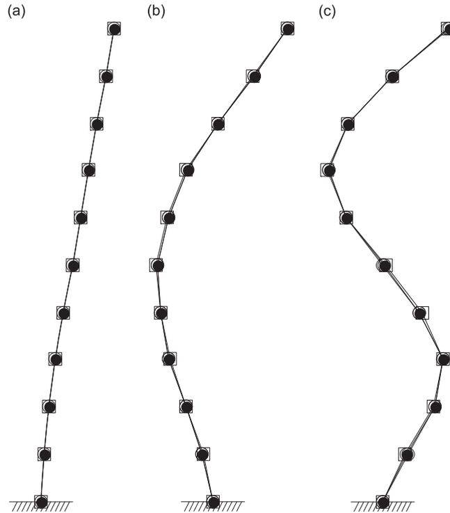
Fig. 17. Mode shapes for (a) the first mode, (b) the second mode and (c) the third mode.
