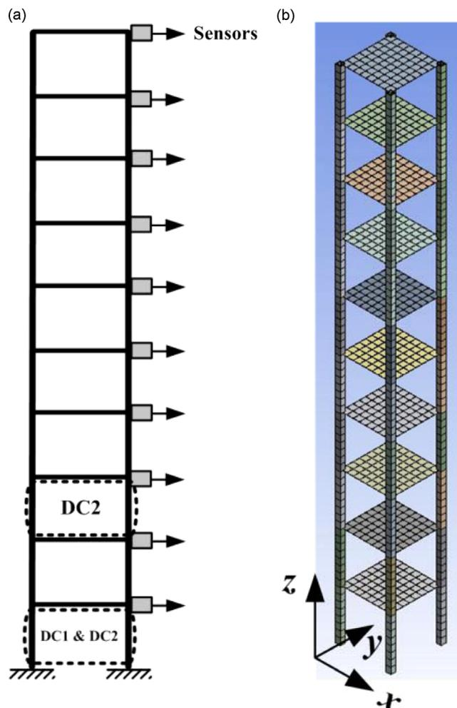
**Fig. 6.** Numerical model (a) damage locations and assumed sensors and (b) ANSYS model.
