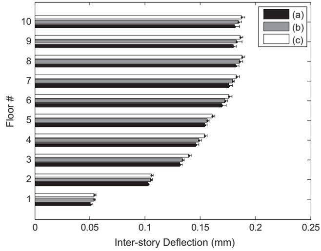
Fig. 19. Inter-storey deflections with  $2\sigma$  deviations (a) IC, (b) DC1 and (c) DC2.
