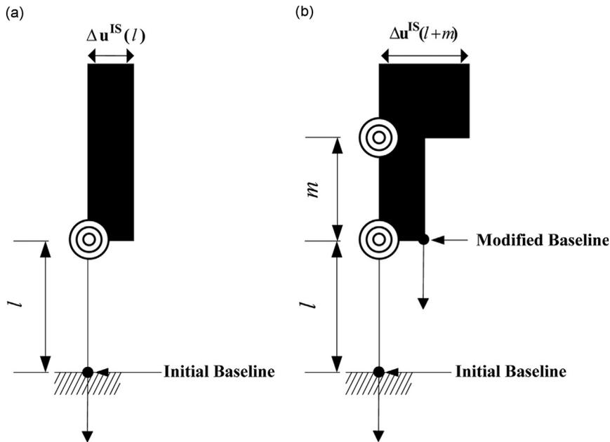
Fig. 3. Multiple damage detection through baseline modification (a) initial baseline and (b) modified baseline.
