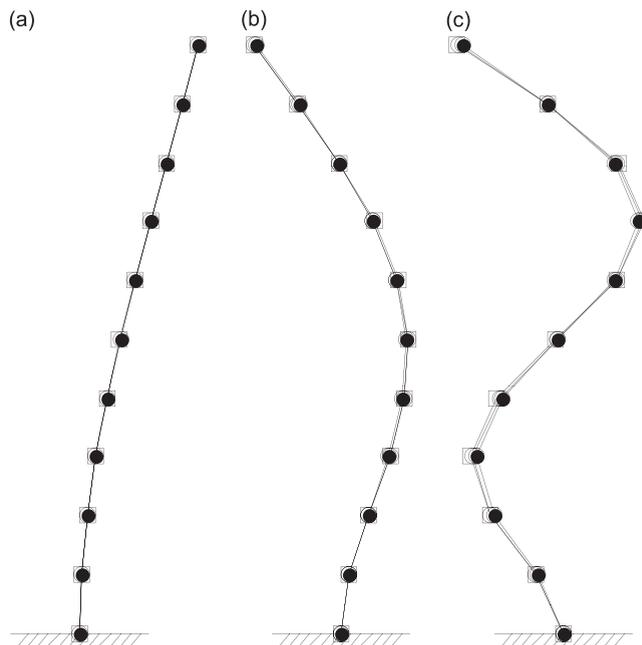
**Fig. 8.** Mode shapes for (a) the first mode, (b) the second mode and (c) the third mode.
