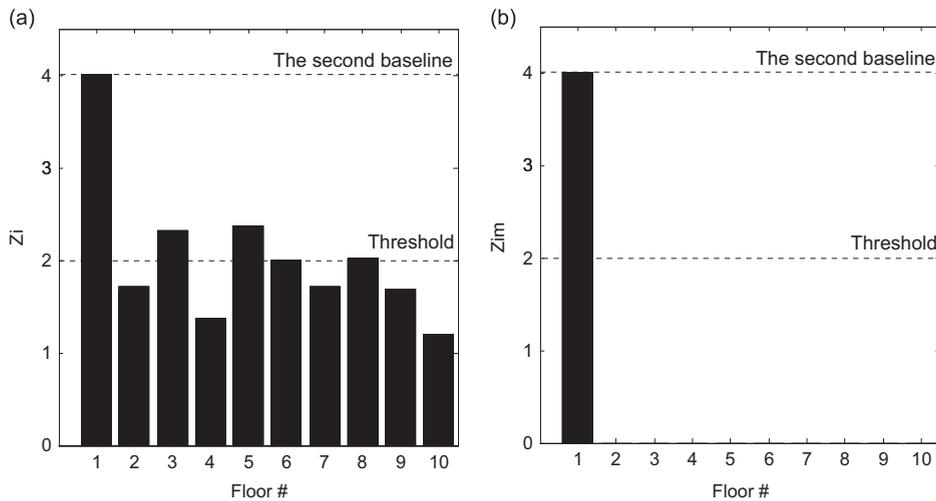
Fig. 21. Damage detection results for DC1 (a)  $Z_i$  and (b) Modified  $Z_i$  ( $Z_{im}$ ).
