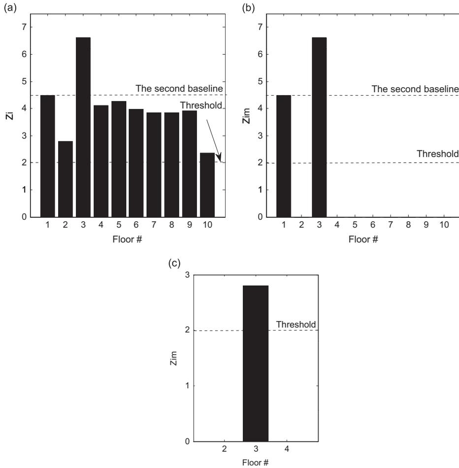
Fig. 22. Damage detection results for DC2 (a) Zi, (b) Modified Zi ( $Z_{im}$ ) and (c) Modified Zi ( $Z_{im}$ ) estimated from the second baseline.
