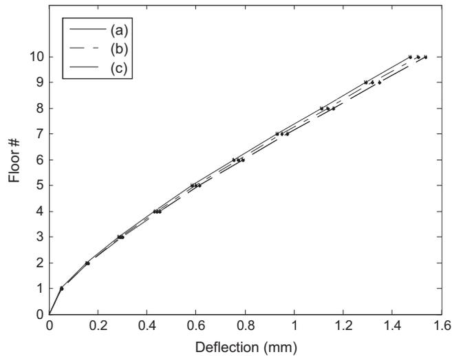
Fig. 18. Deflections with  $1\sigma$  deviations (a) IC, (b) DC1, and (c) DC2.
