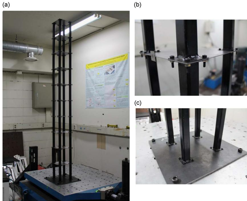
Fig. 13. (a) Experimental model, (b) structural boundary condition and (c) connection between columns and floors.
