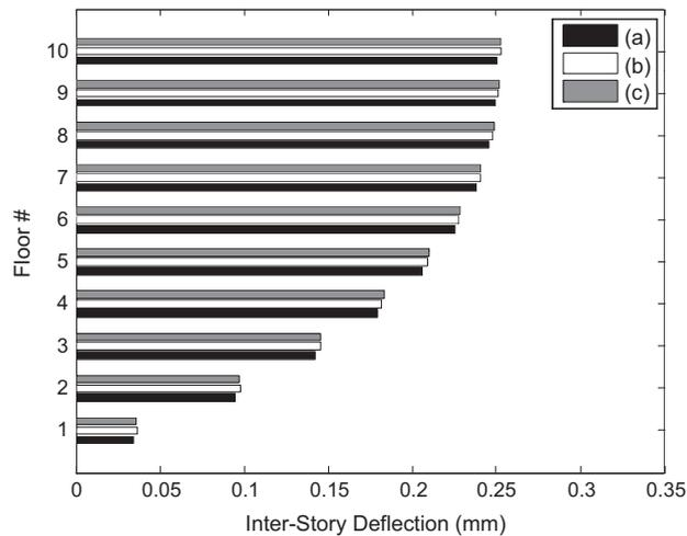
Fig. 10. Inter-storey deflections (a) IC, (b) DC1 and (c) DC2.
