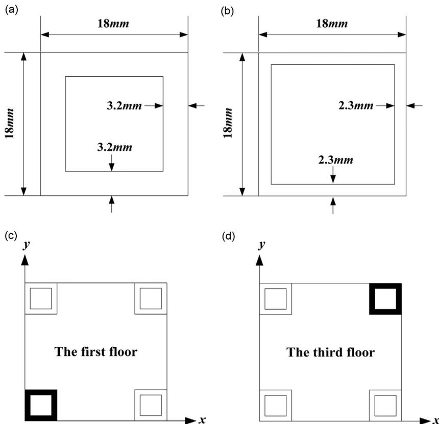
Fig. 7. Damage scenarios (a) intact column, (b) damage column, (c) damage column on the first floor (top view) and (d) damage column on the third floor (top view).
