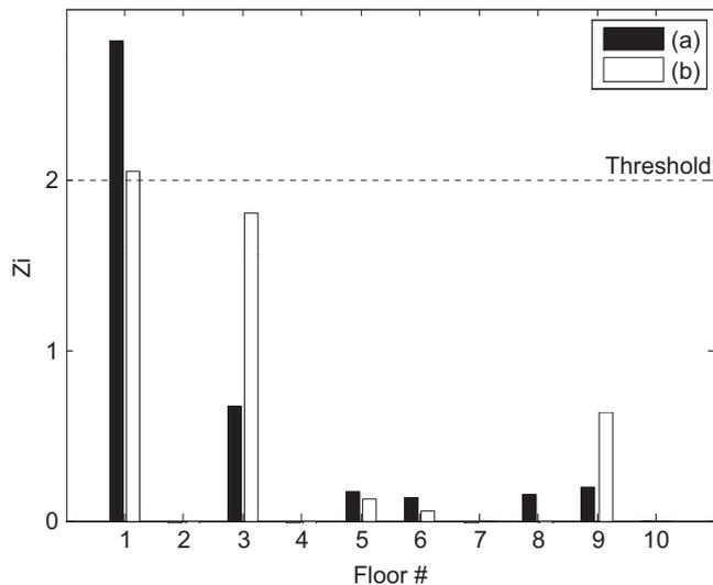
Fig. 24. Investigation of the damage location(s) by ULS curvatures approach (a) DC1 and (b) DC2.
