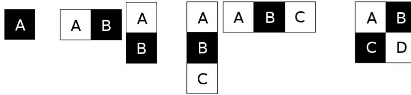
**Figure 1: Haar-like features.** The feature values are calculated by subtracting sums of pixel intensities in neighbouring rectangular regions A, B, C, D. Position and scale of features on images are important.
