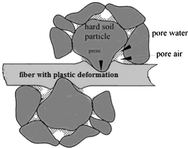
Fig. 8. Sketch drawing of contact condition between hard soil particles and fiber surface under press (modified from Tang et al., 2010).
