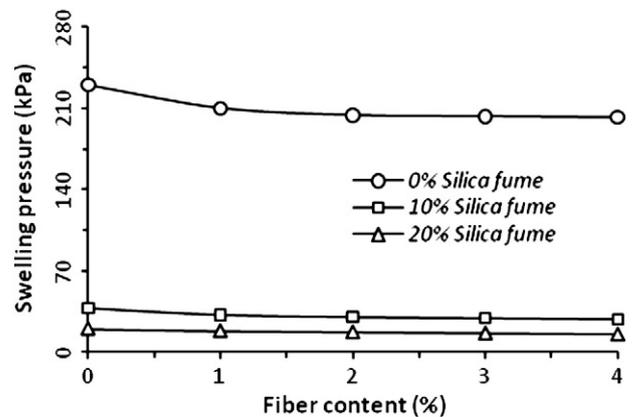
**Fig. 13.** Effect of the silica fume and scrap tire rubber fiber on the swelling pressure.
