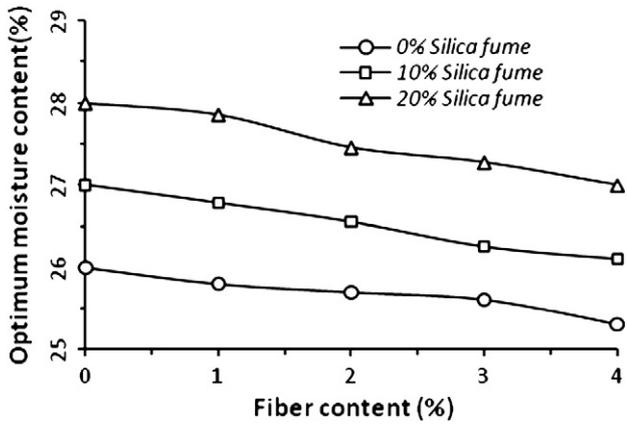
Fig. 4. Effect of the scrap tire rubber fiber on the optimum moisture content.
