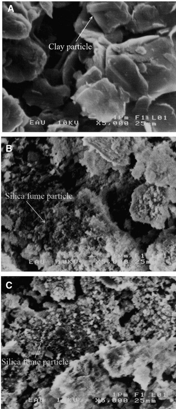
Fig. 14. Images of silica fume-modified clayey soil with (A) 0% silica fume, (B) 10% silica fume and (C) 20% silica fume.
