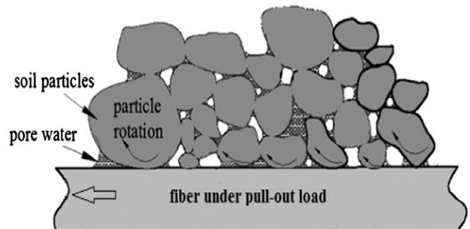
Fig. 7. Sketch drawing of interfacial mechanical interactions between soil particles and fiber (modified from Tang et al., 2010).
