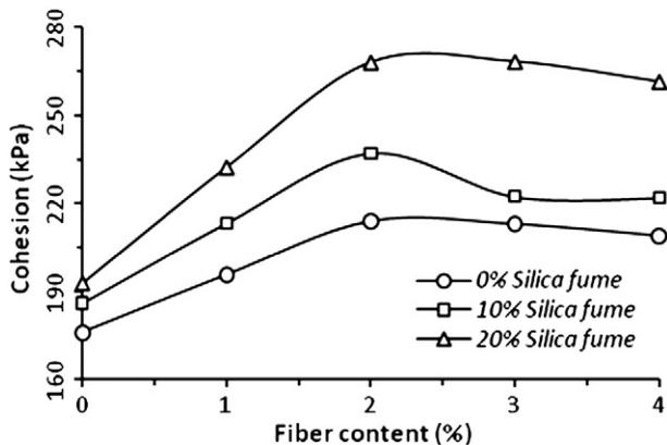
Fig. 9. Effect of the scrap tire rubber fiber on the cohesion.
