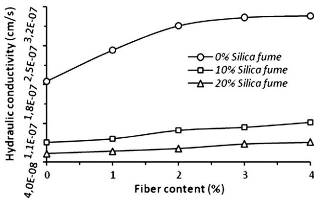
**Fig. 12.** Effect of the silica fume and fiber on the hydraulic conductivity.
