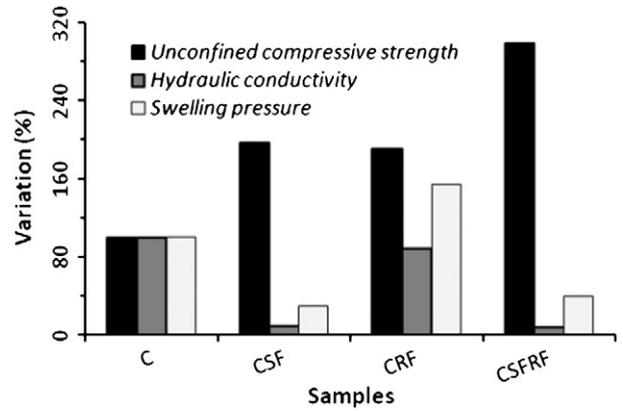
Fig. 6. Variation of UCS, swelling pressure and hydraulic conductivity with the silica fume, fiber and silica fume–fiber mixtures.
