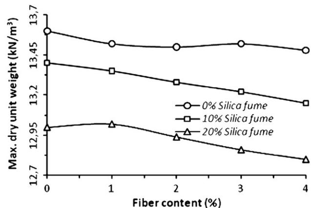
Fig. 3. Effect of the scrap tire rubber fiber on the maximum dry unit weight.
