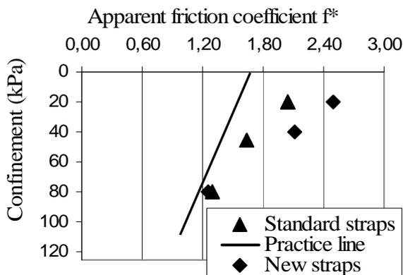
Figure 5. Improvement of the apparent friction coefficient with the new straps in the gravel.
