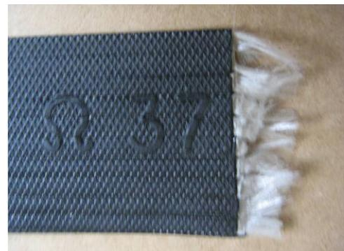
Figure 1. Standard GeoStrap design
