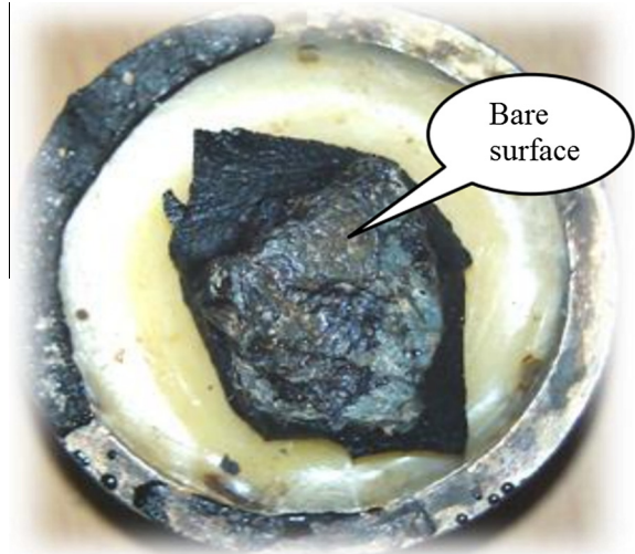
Fig. 6. The failure state of damp sample.
