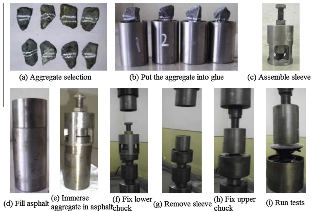
Fig. 2. The procedure of pull-off test.
