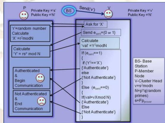
Fig. 3. Post deployment Phase of Implementation of ZKP in our Proposed Scheme
