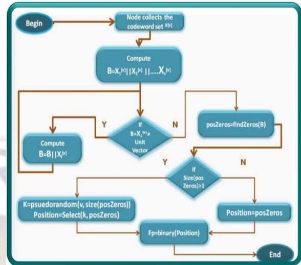
Fig. 2. Predeployment Phase of Model for Generation of Fingerprint
