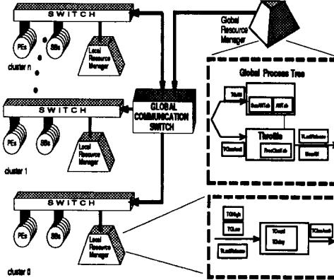
Figure 1: Massively Parallel System with Centralised Throttle Control
