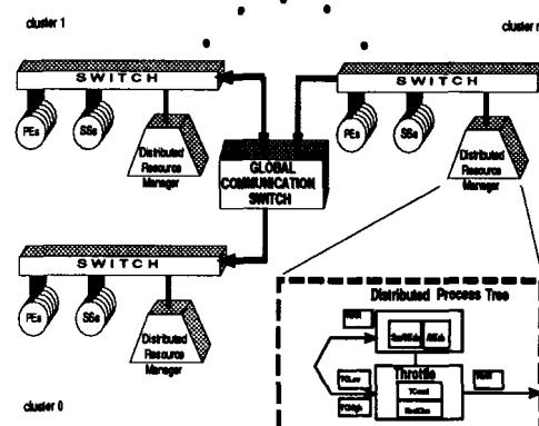
Figure 3: Massively Parallel System with Distributed Throttle Control
