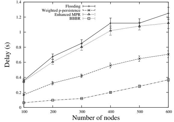
Fig. 10. End-to-end delay for various numbers of nodes.
