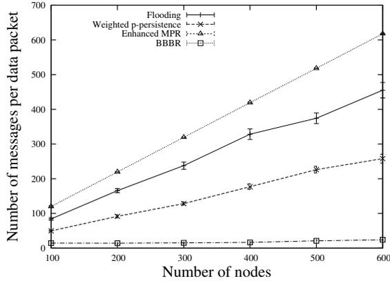
Fig. 8. Number of messages per data packet for various numbers of nodes.
