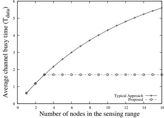
Fig. 6. Channel busy time for various number of nodes in the sensing range.
