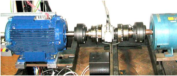
Fig. 1. Prototype BDFM machine (left) on test rig with torque transducer and DC load machine (right)
