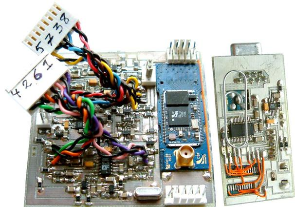
Fig. 4. Two electronic boards constructed for instrumenting the BDFM rotor. Left: Electronic circuitry mounted on the rotor shaft. Right: Electronic circuitry designed for logging data
