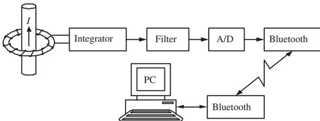
Fig. 2. Functional block diagram of the rotor instrumentation system
