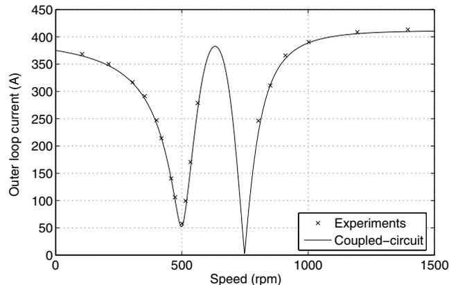
Fig. 10. Rotor outer-loop current in the cascade mode of operation.
