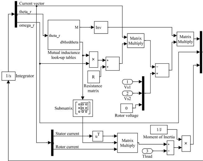
Fig. 6. The BDFM coupled-circuit model implementation in Simulink
