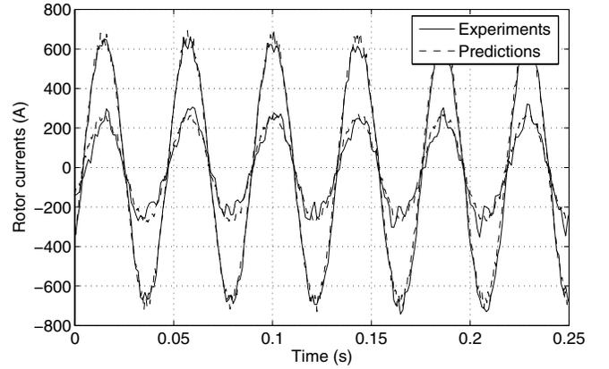
Fig. 7. Middle and inner loop currents within one nest for the nested-loop rotor. The middle loop current clearly has a greater amplitude.
