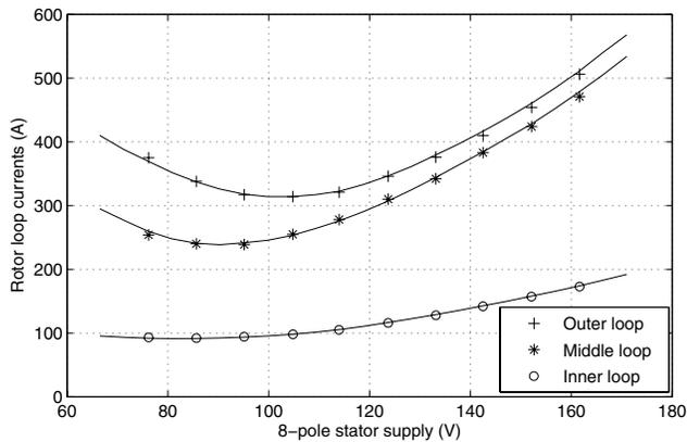
Fig. 9. The rotor loop currents at synchronous mode of operation. Solid lines are the coupled-circuit predictions and marks indicate the experimental results.
