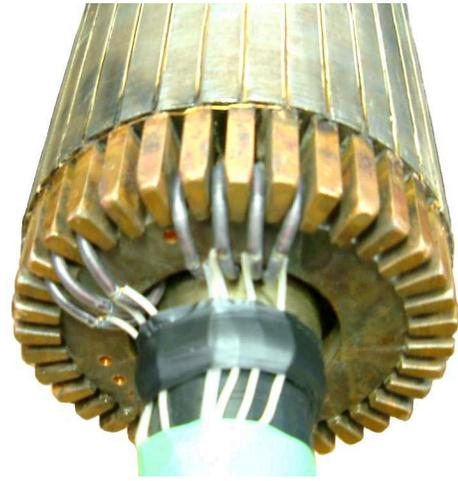
Fig. 3. Rogowski coils installed on the nested-loop prototype rotor to measure end-ring currents
