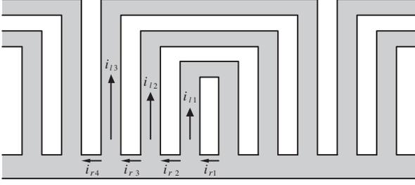
Fig. 5. End-ring and bar currents in a nested-loop rotor design
