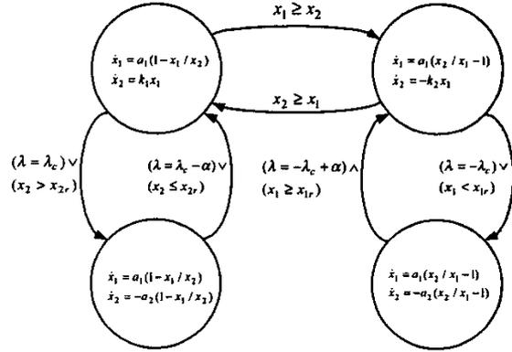
Fig. 7. Automaton diagram of the proposed control system.
