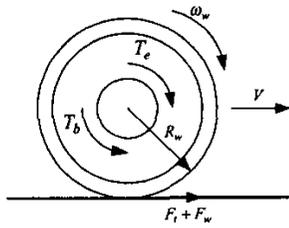
Fig. 1. Wheel diagram [7].
