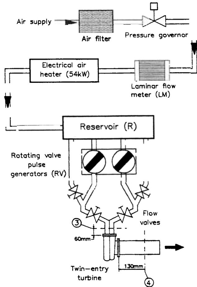
Fig. 1 Arrangement of the turbine feeding line on the test facility.
