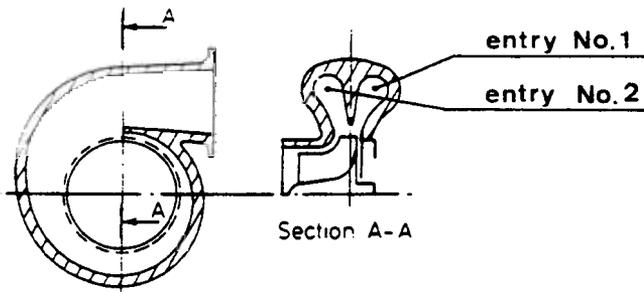
Fig. 2 - Schematic of a twin-entry radial turbine.
