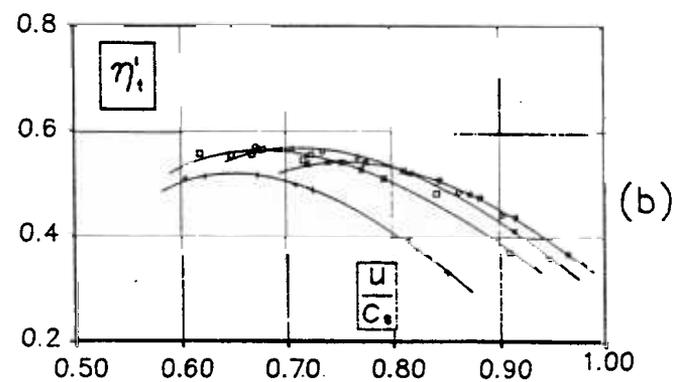
Fig. 3 - Single and twin-entry (full admission) turbine mass flow (a) and efficiency (b) characteristics.
