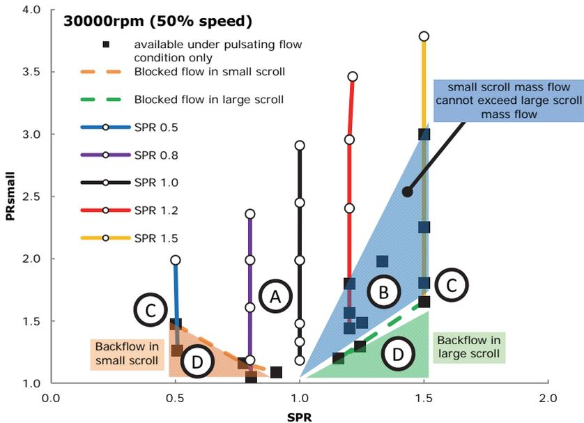
**Figure 6: Small turbine volute flow interaction:**
