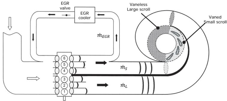
**Figure 2: The system of the Asymmetric double-entry turbine with a 6-cylinders engine**
