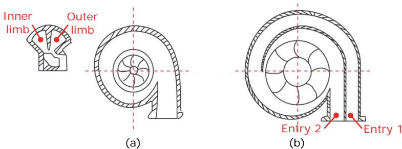
**Figure 1: Comparison between multiple-entry turbine designs (1): (a) Twin-entry and (b) Double-entry turbine design**
