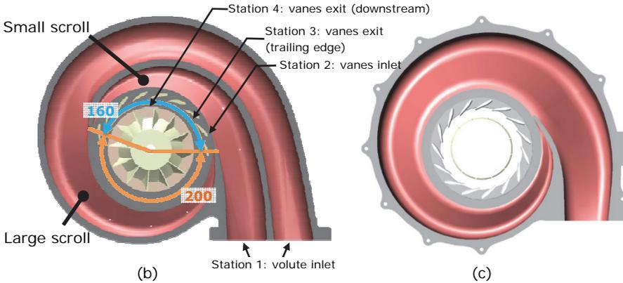
**Figure 4: Asymmetric double-entry turbine volutes A/R design**
