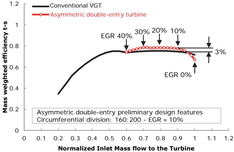
**Figure 3: The turbine efficiency advantage of asymmetric double-entry turbine against conventional VGT when EGR is being operated widely (The mass flow was normalized with the design-point mass flow rate of the single-entry VGT used for comparison)**
