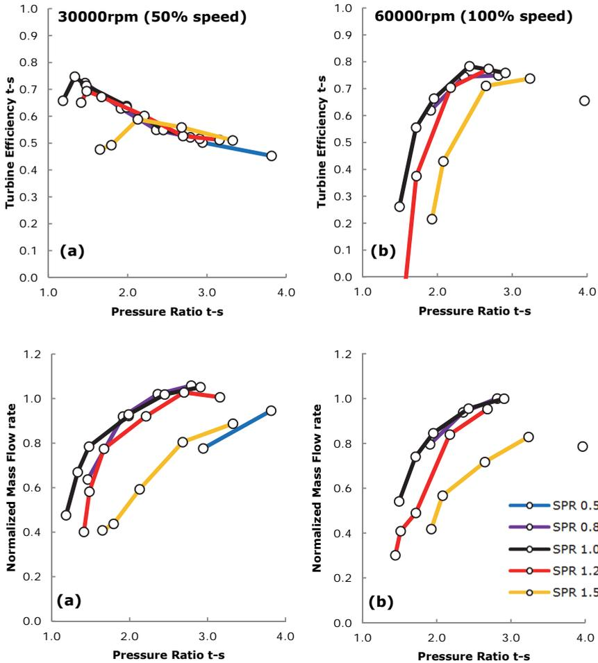
**Figure 5: Turbine performance of the Asymmetric double entry turbine at**
