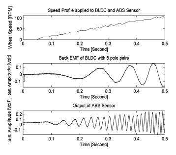
Fig. 4. Comparison between a 48-tooth ABS sensor (made by Repco Ltd.) output and BLDC motor (with eight-pole pair) back EMF.
