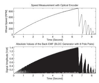
Fig. 12. Top: Reference (optical encoder) measurements. Bottom: Absolute values of the back-EMF signal shown in Fig. 11.
