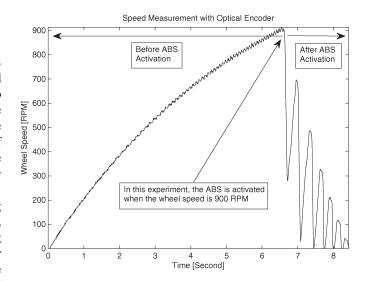
Fig. 8. Typical reference wheel speed measurements by optical encoder during a complete experiment.
