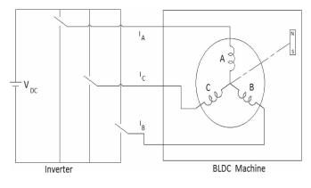
Fig. 2. Electronically commutated BLDC motor.
