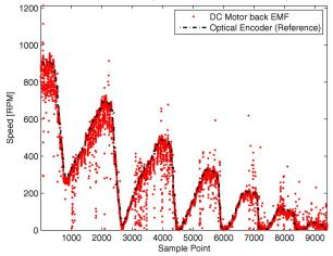
Fig. 16. DC-motor back-EMF speed measurement.
