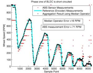
Fig. 15. Result of aggregating wheel speed measurements (using the amplitude method) by median operator.
