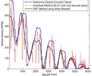
Fig. 14. Wheel speed estimation from EMF of a BLDC with only two pole pairs using the DWT method.
