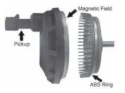
Fig. 1. Commercial ABS sensor (made by Repco Ltd.) used in sedan cars.
