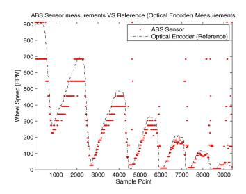
Fig. 10. Comparison between ABS sensor measurements and reference (optical encoder) measurements during ABS activation.
