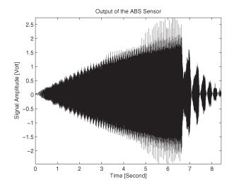
Fig. 9. Unprocessed output of ABS sensor corresponding to Fig. 8.
