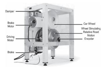
Fig. 6. Standard ABS setup (made by Inteco) for frictional brakes [27].
