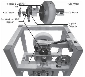
Fig. 7. Installation details of the modified ABS test rig for realizing the sensorless ABS.
