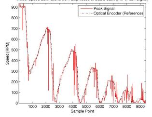
Fig. 13. Peak signal (wheel speed estimations using the amplitude method) corresponding to the amplitude signal shown in Fig. 12.
