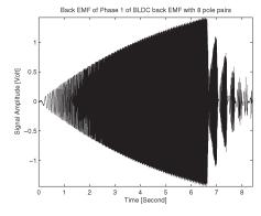
Fig. 11. BLDC Back EMF (with eight pole pairs) corresponding to Fig. 8.
