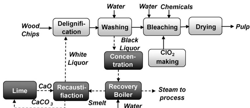
Fig. 1 – Simplified diagram of the Kraft process.
