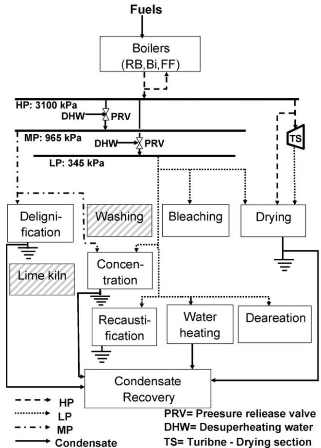
**Fig. 6 – Simplified diagram of the production, utilization and post-utilization of steam.**
