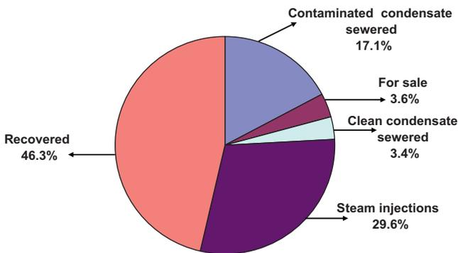
**Fig. 4 – Distribution of condensates in the process.**
