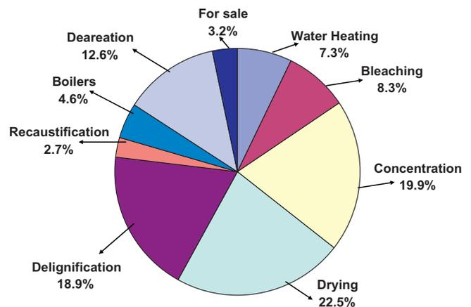
Fig. 3 – Energy consumed by process department as a fraction of the total consumption.
