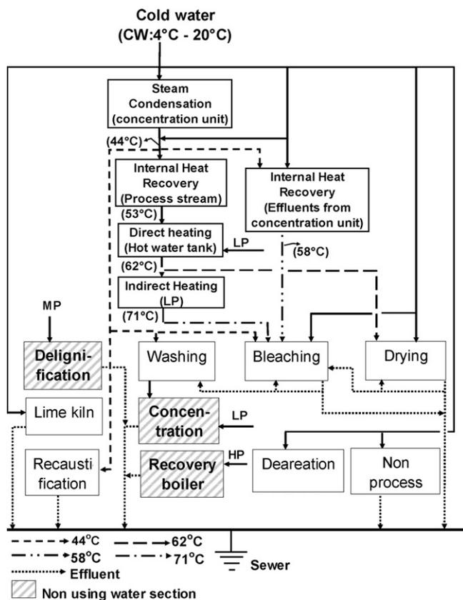
Fig. 9 – Simplified diagram of the production, utilization and post-utilization of water.
