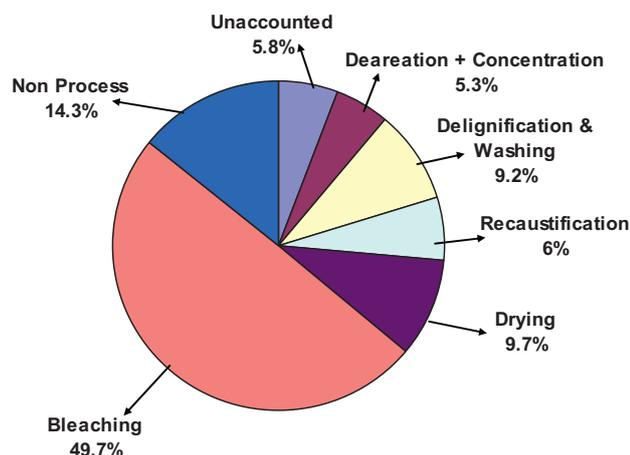
Fig. 7 – Water consumption distribution in the process.
