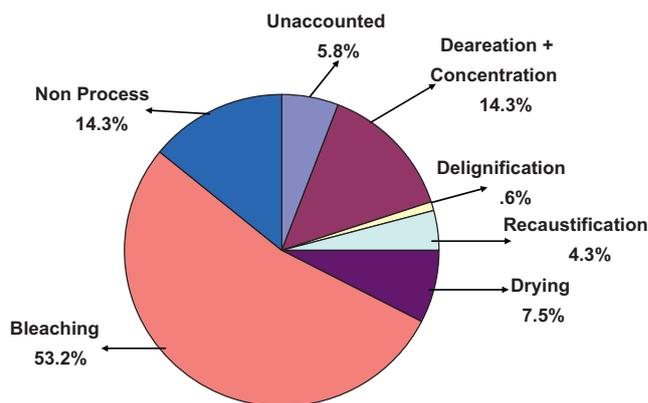
Fig. 8 – Distribution of sewerred effluents in the process.
