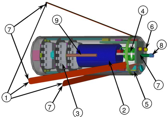
Fig. 10. Conceptual assembly of a swimming micro robot for neurosurgery. The components of the robot are: 1) Three swimming tails, 2) Power source (here 5 Renata ZA10 batteries in series), 3) Packaged IC for command control and communication, 4) Antenna, 5) Endoscopic Camera, 6) LEDs, 7) Force sensors, 8) Tool for intervention, 9) Localization sensor (here an Aurora magnetic tracker receiving coil).
