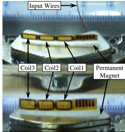
Fig. 5. Image of the experimental magnetic tail. The image shows the tail from two points of view: profile (lower image; reflection from the vessel wall) and half profile (upper image; direct image trough the water).
