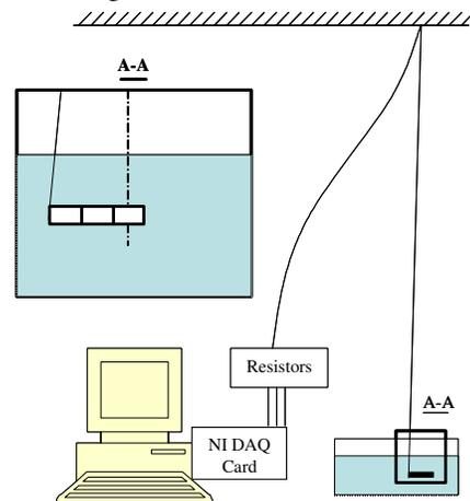
Fig. 6. Illustration of the setup of the swimming experiments.
