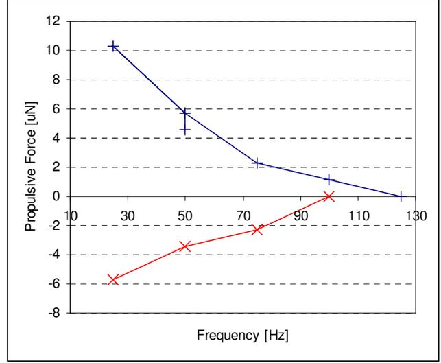
Fig. 8. Propulsive force versus frequency in forward (blue line with plus markers) and backward (red line with x markers) swimming of the magnetic swimming tail.
