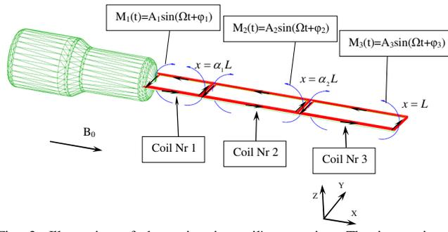
Fig. 3. Illustration of the swimming tail's operation. The interaction between the  $B_0$  constant magnetic field in the  $x$  direction and three alternating currents in three coils, (the direction of the current in each coil is denoted by a black arrow) in the  $y$  direction creates alternating bending moments in the  $z$  direction. The moments have the same frequencies but different phases and amplitudes as shown.
