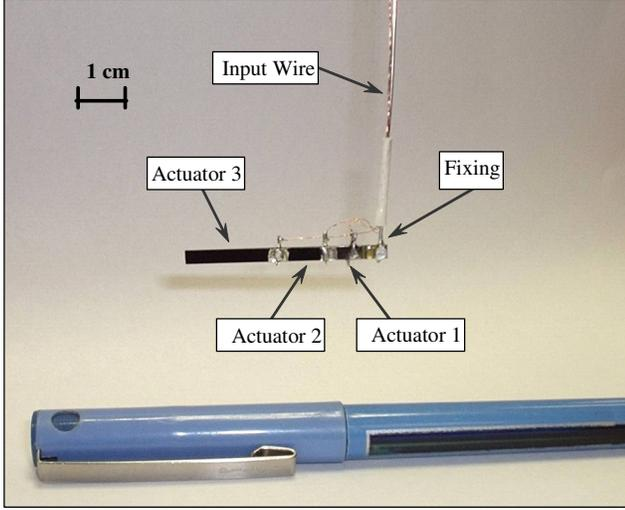
Fig. 2. A commercial piezoelectric bimorph (APC 40-1055) divided into three sections (Actuator 1-3) designed to create swimming.
