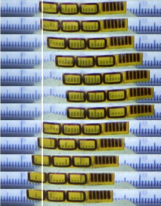
Fig. 7. Swimming of the magnetic tail forward (the upper 7 images) and backward (the lower 5 images). The vertical white line denotes the initial location of the tail.
