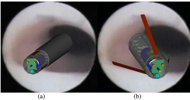
Fig. 9. Illustration of the swimming micro robot a) inserted by a cannula into the lateral ventricle and b) swimming to its target area. The background has been generated from an endoscopic image of the lateral ventricles.
