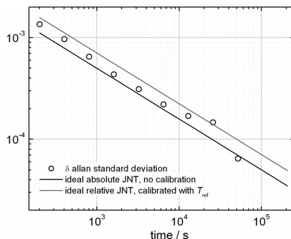
**Figure 6.** Allan standard deviation of the JNT error  $\delta_j = \Delta T^j / T_{90}$  compared with the corresponding theoretical predictions for an ideal absolute thermometer and an ideal relative thermometer calibrated against a reference temperature  $T_{\text{ref}}$ .
