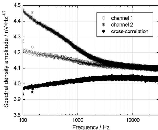
**Figure 5.** Amplitude spectra of the cross-correlation signal  $N(f_k)$  and of the autocorrelation of the two spectrum analyzer acquisition channels separately. The flicker noise of A is apparent in the autospectra. The shape of  $N(f_k)$  is slightly convex because of the bandpass filtering in the second stage of A.
