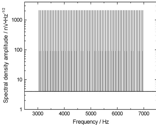
**Figure 3.** The calibration signal  $e_C$  for a bandwidth  $B = 3$  kHz to 7 kHz. The baseline is the Johnson noise  $e_N$ .
